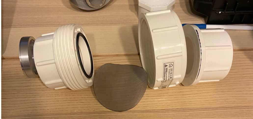
Figure 36. Filtration System Laid Out
