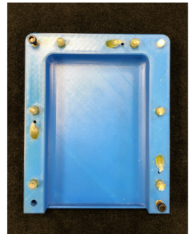
Figure 5: The figure shows the ZFrame used on the Neuro-Robot for registration.
