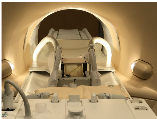
Figure 24: The figure shows the AAMP Phantom used during the NeuroRobot Targeting Tests.
