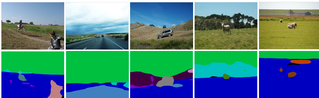
Figure 5.3: Some Semantic segmentation results using Early Supervision Full Convolutional Network (ES-FCN), where blue represents the grass, green represents the sky, light blue represents the ground and other colors represent other specific objects (referencing the object color corresponding to the list in PASCAL-Context Dataset[39])
