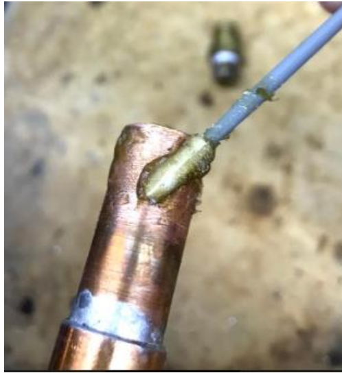
Figure 16: Paste flux application
