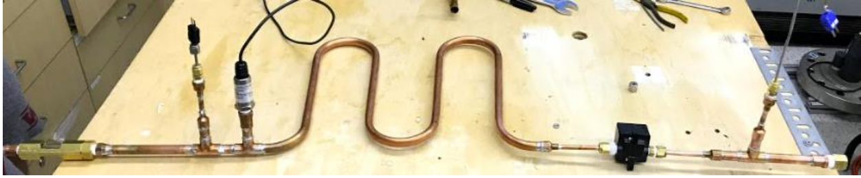
Figure 20: Evaporator with instruments added
