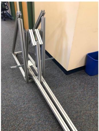
Figure 23: Assembled fourbar and skid frame
