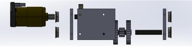
Pulley Gearbox: Exploded side view
