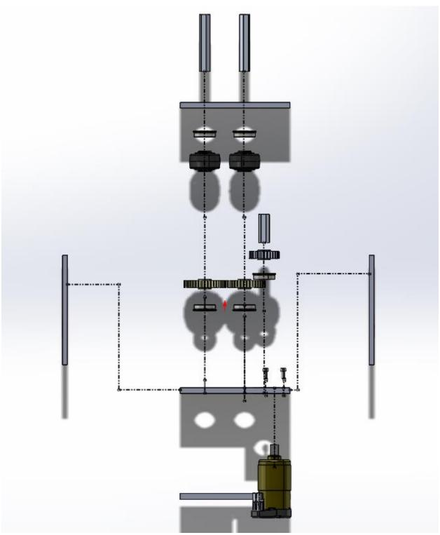
Gripper Gearbox: Exploded top view
