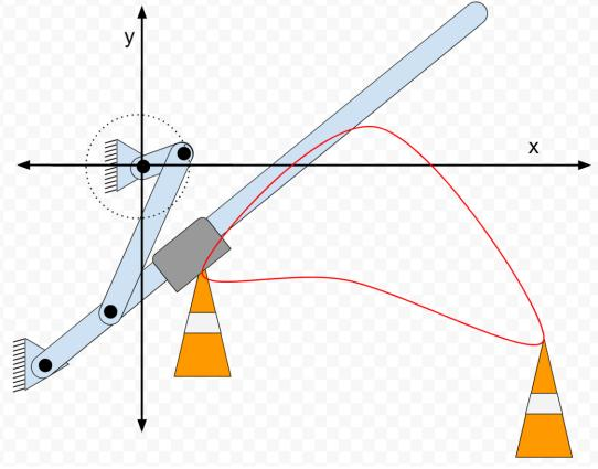
Figure 19f: Computer generated image with coupler curve
