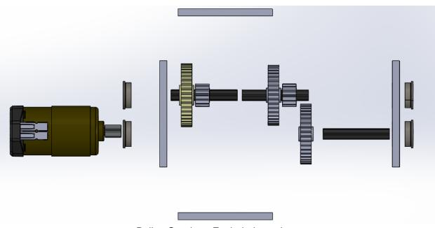
Pulley Gearbox: Exploded top view
