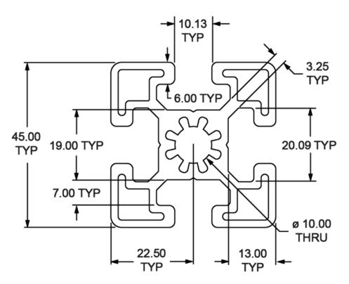
Figure 8: 45 x 45 mm stock profile dimensions
