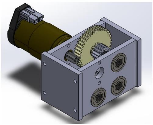
Figure 16a: Pulley gearbox isometric view
