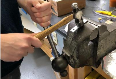
Figure 21: Hammering a bracket to make an acute angle
