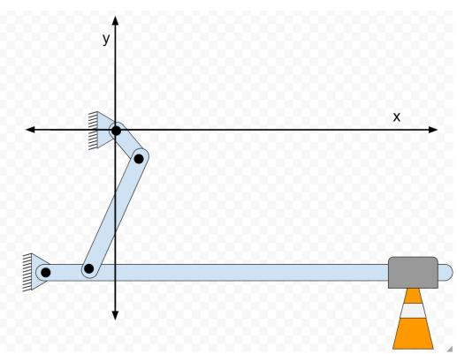
Figure 19c: Step 2- Place Cone: The coupler is lowered and the gripper is pulled in the positive x direction.
