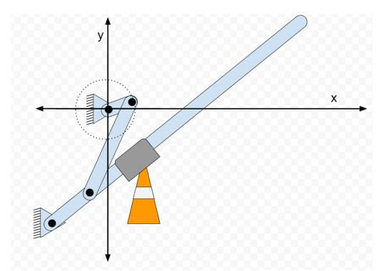
Figure 19b: Step 1- Grip Cone: The coupler is raised and the gripper is pulled in the negative x direction.
