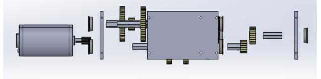
Main Gearbox: Exploded side view
