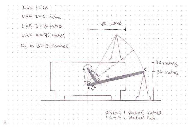
Figure 4: Hand drawing of early linkage concept
