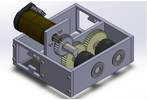
Figure 15a: Gripper isometric view
