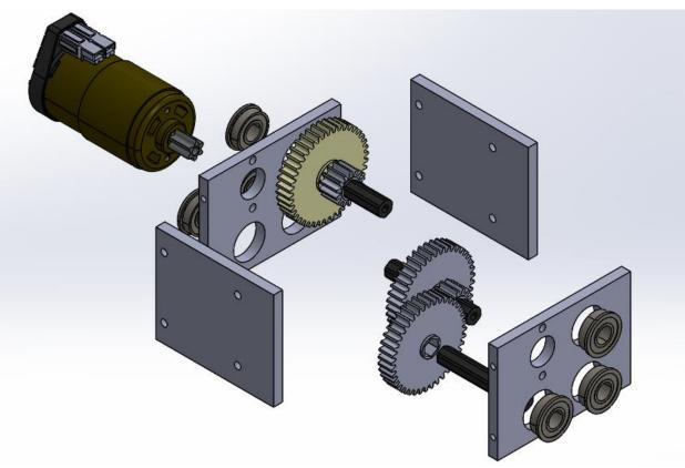
Pulley Gearbox: Exploded isometric view
