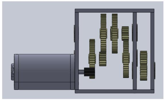
Figure 17a: Gearbox side view
