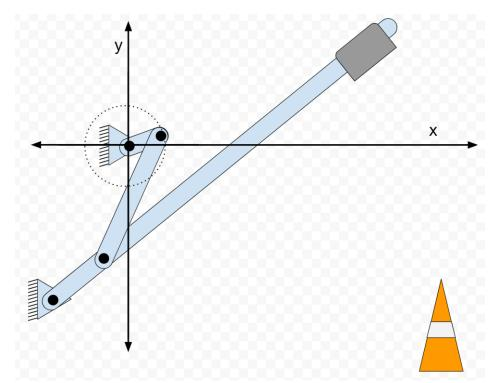
Figure 19d: Step 3- Drop Cone and Raise fourbar: The cone is released and the coupler is raised.
