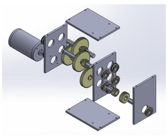
Main Gearbox: Exploded Isometric View
