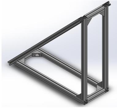
Figure 14a: Skid frame isometric view
