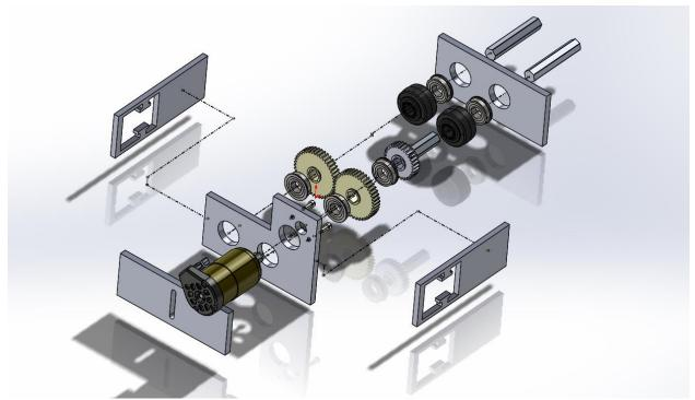
Gripper Gearbox: Exploded isometric view
