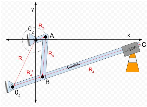
Figure 19a: Motion diagram with labels
