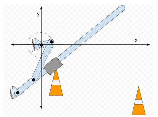
Figure 19e: Step 4- Grip Next Cone: Equivalent to step 1, the coupler stays raised and the gripper is pulled in the negative x direction. The cycle repeats.
