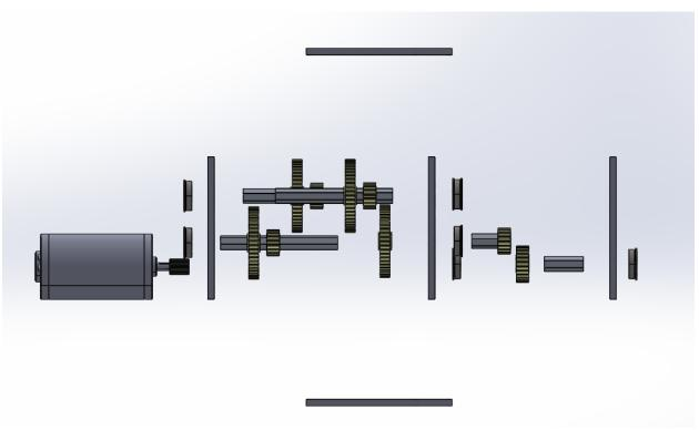
Main Gearbox: Exploded top view
