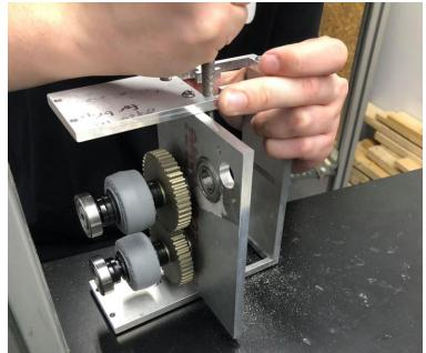
Figure 24: Filing the gripper gearbox
