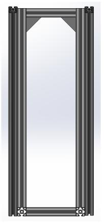
Figure 14c: Skid frame front view
