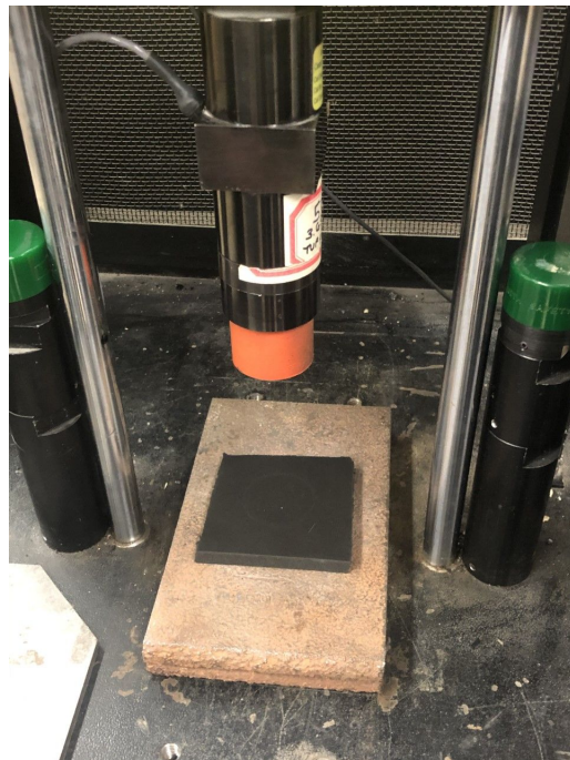
Fig. 21: Instron 9400 Series Drop Tower setup close view
