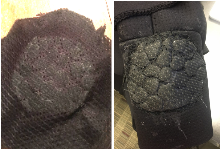
Fig. 24: Side delt pad construction
