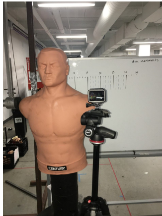
Fig. 30: Baseline impact test setup
