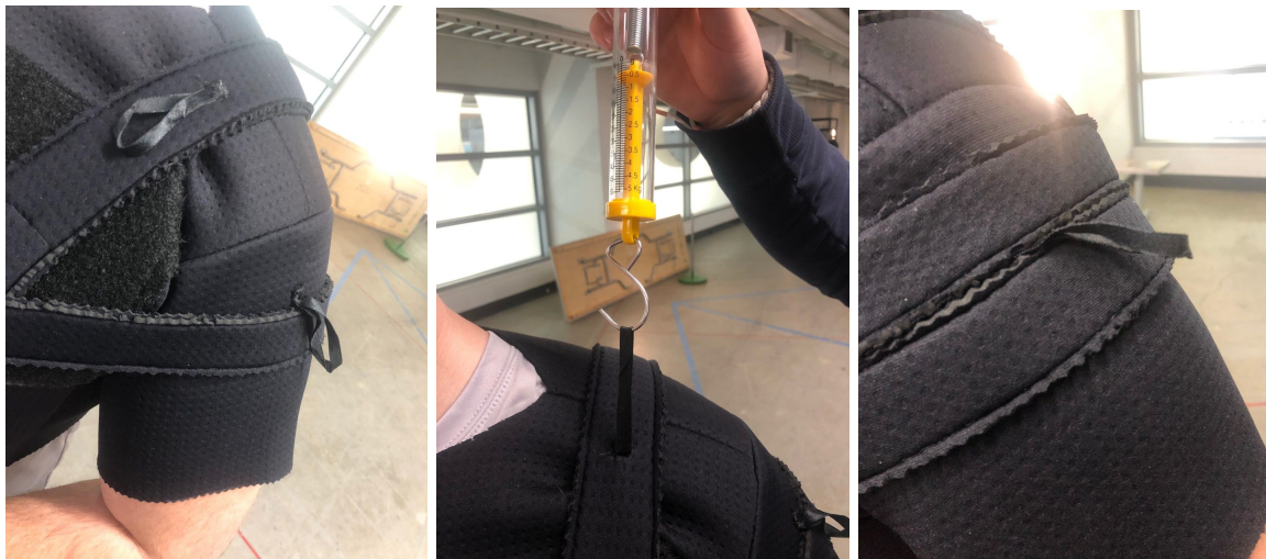
Fig. 31: Pull loops on brace, and AC compression test
