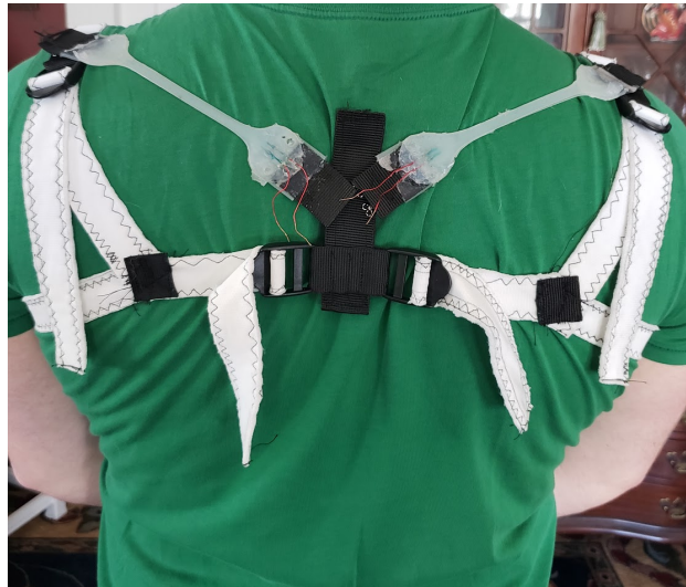
Figure 30: The harness on a human's back with the sensors mounted.
