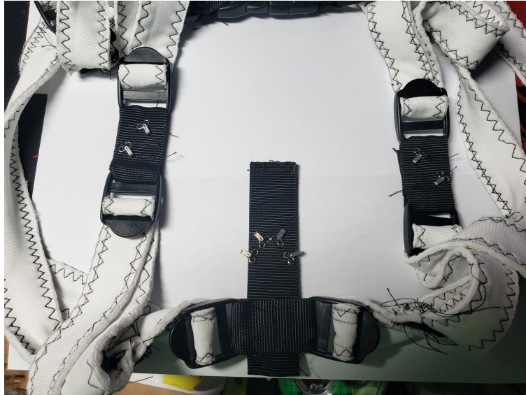
Figure 29: The spine and shoulder assemblies with hooks attached
