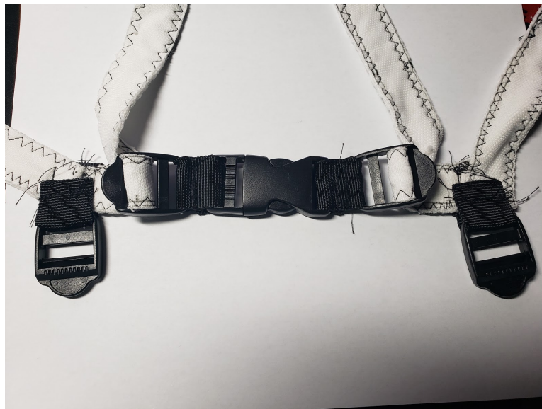
Figure 23: The assembly of the buckle and front-arm assemblies.
