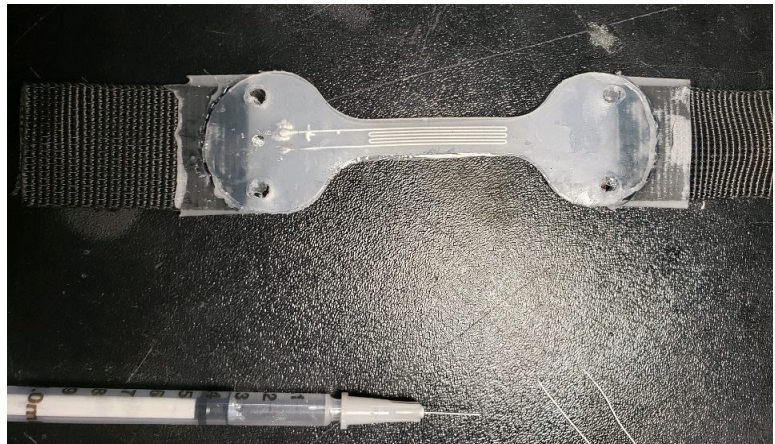
Figure 7: Final manufactured sensor, with no stiffness gradient.
