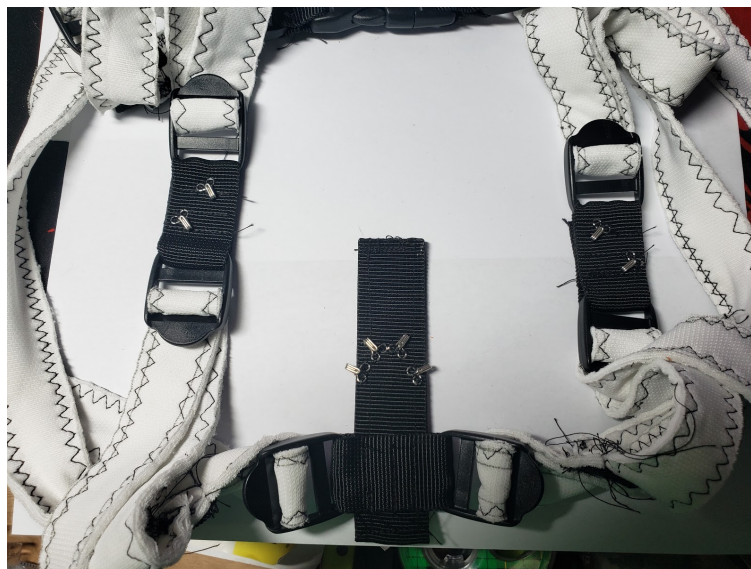
Figure 16: The spine and shoulder assemblies with hooks attached
