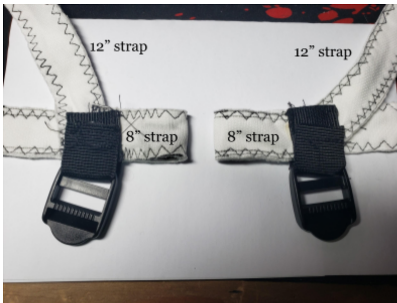
Figure 21: The front-arm assemblies, with straps labeled.
