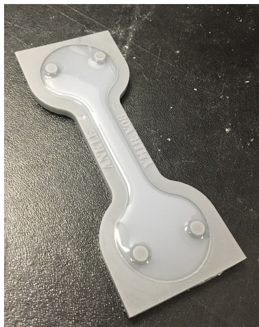
Figure 9: silicone curing in mold
