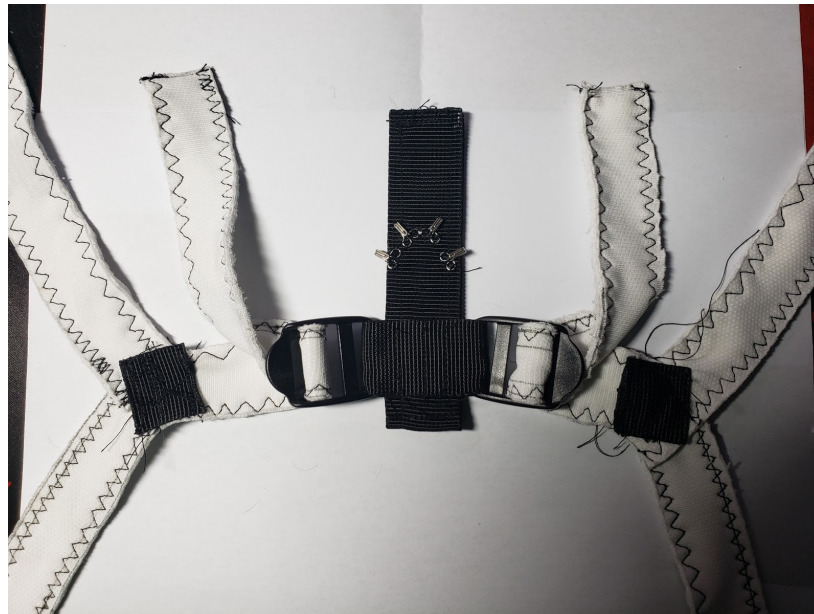
Figure 25: The assembly of the spine and back-arm assemblies.
