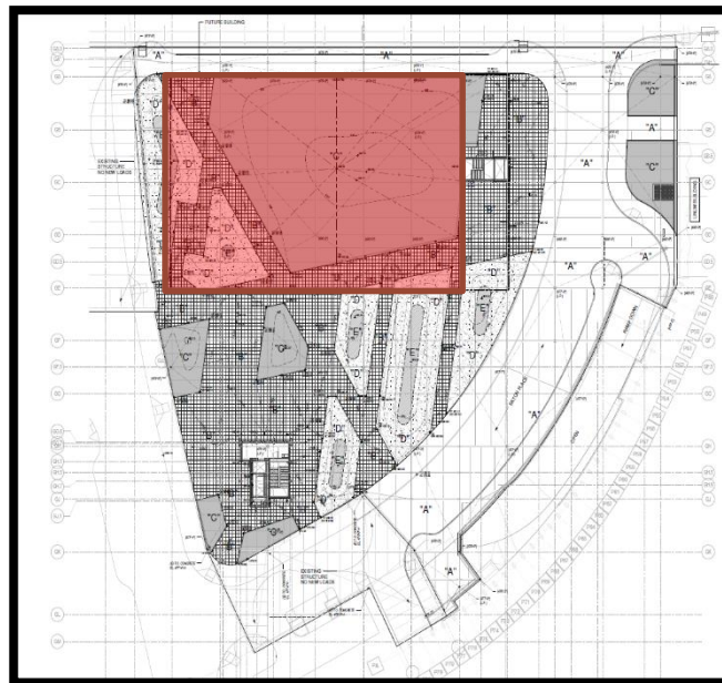
Figure 25 - Loading Conditions at the Plaza Level with Area of Interest Highlighted in red. (Gateway)
