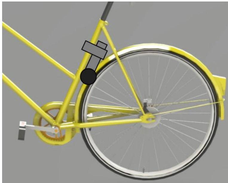
Figure 5.7: Tire Top Generator Concept
