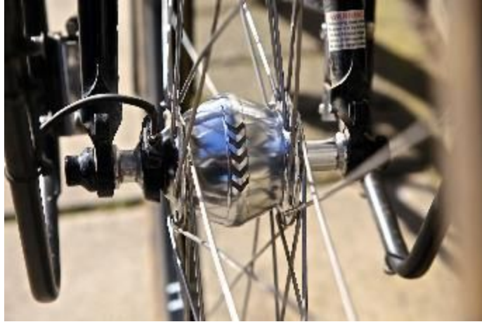
Figure 2.14: Hub Dynamo (SP Dynamo Hub PV-8 Review, 2015)
