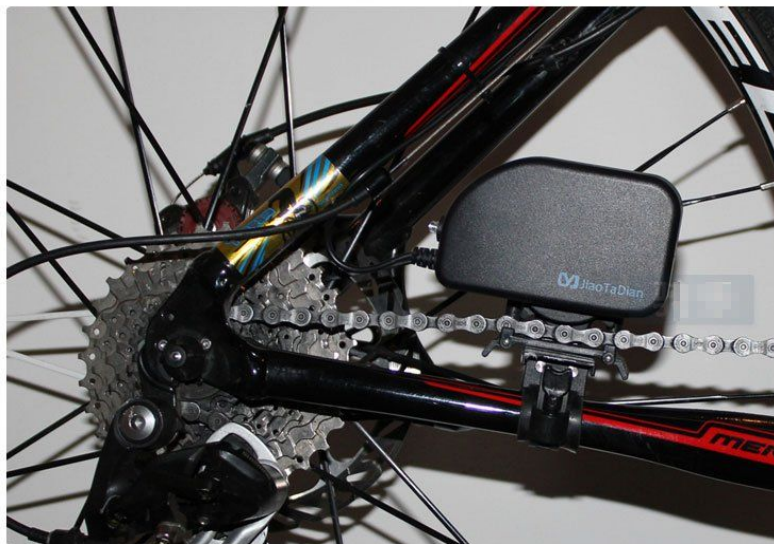
Figure 2.16: Chain-Driven Dynamo (Outdoor Portable Charger Bike Generator-Chain Type, n.d.)
