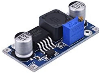
Figure 6.7: DC/DC Boost Converter Module XL6009
