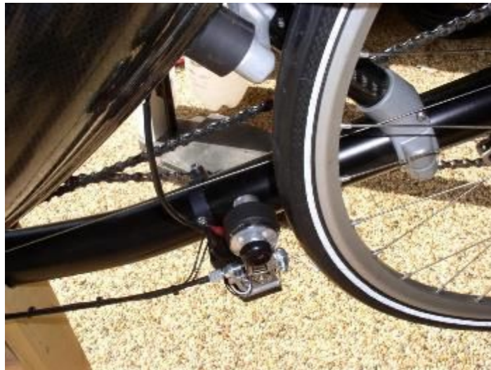
Figure 2.15: Bottom Bracket Dynamo (Dynamo Hub on Trike, 2011)
