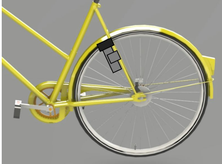
Figure 5.6: Tire Sidewall Generator Concept
