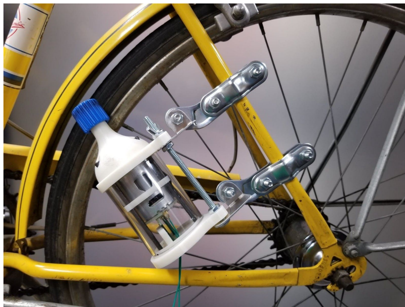
Figure 7.3: Prototype Generator Mounted on Bicycle
