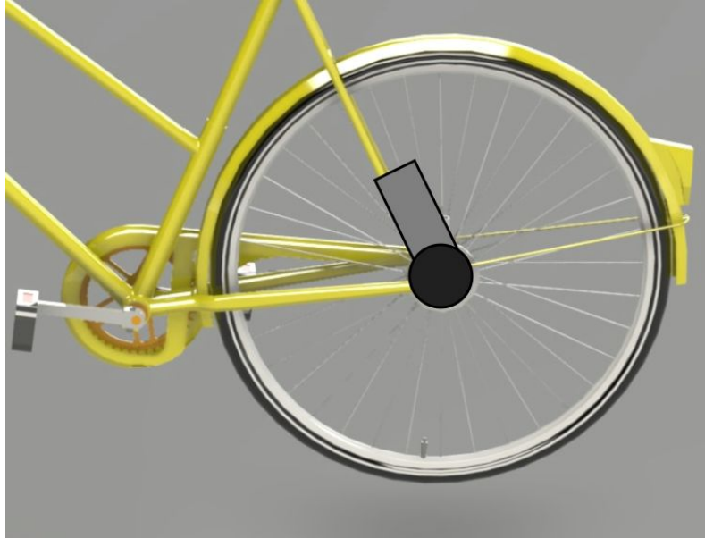
Figure 5.9: Generator that Interfaces with Spokes Concept
