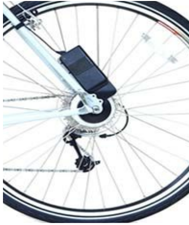
Figure 2.17: Wheel-Mounted Dynamo (Dynamo Chargers Outside of the Hub, n.d.)
