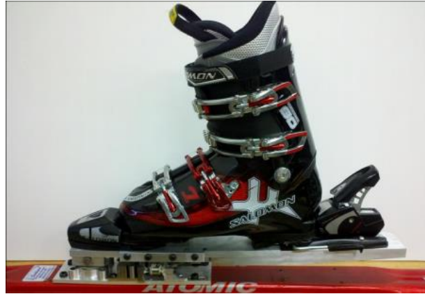
Figure 3: The physical integration of the ACL injury reducing binding plate MQP (Austin, Ferland, & Seibold, 2011).
