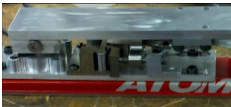
Figure 4: A look at the mechanism of the ACL injury reducing binding plate (Austin, Ferland, & Seibold, 2011). It can be seen that the mechanisms to absorb BIAD loads has been decoupled from the mechanism to absorb phantom foot loads.
