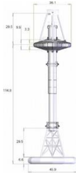
Figure 3: Point Absorber Device (Voorhis, 2012)
