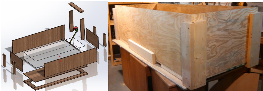
Figure 26 Exploded View and Final Construction of the Wave Tank
