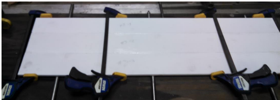
Figure 28 Clamped Tier 1 to Allow Proper Setting of Biscuit Joints
