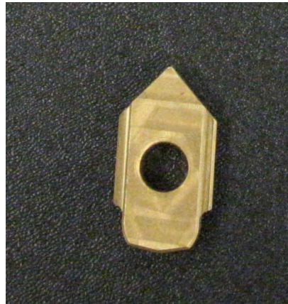
Figure 16: Follower after machining
