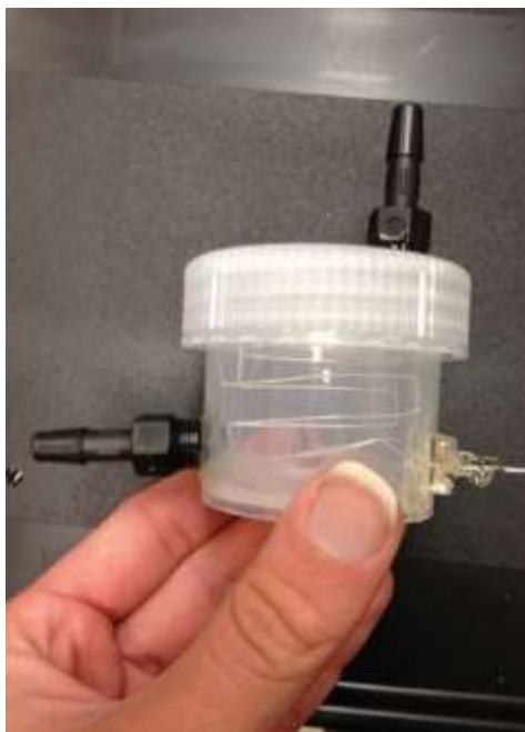
Figure 24: Actual ETC Chamber made from Nalgene Bottle
