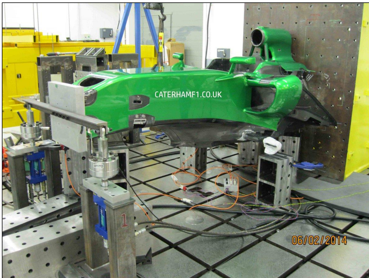
Figure 14: Chassis Stiffness Test Jig
