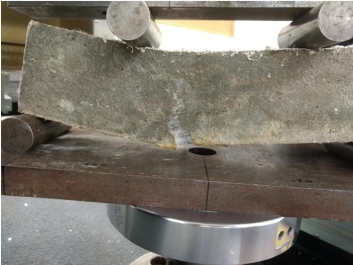
Figure 4.8: A crack formed in Specimen 2
