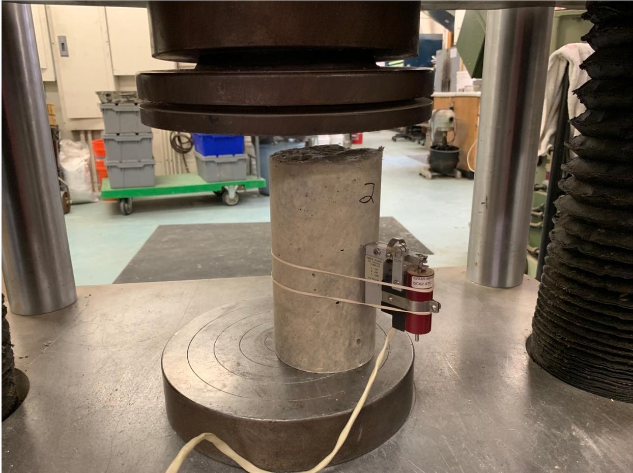
Figure 5.5: Testing Setup for Compressive Testing
