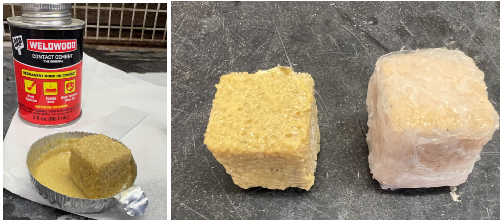
Figure 4-28 Fully dehydrated ECM samples were coated with WELDWOOD Original Contact Cement (yellow) and GE Advanced Silicone (white).
