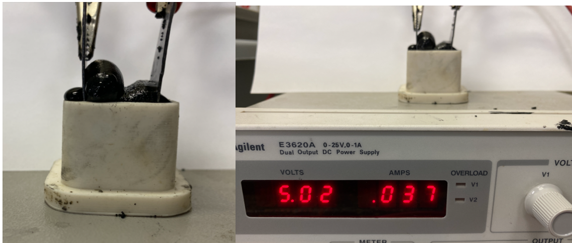
Figure 5-16 The experiment set up of carbon black modified ECM.
