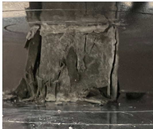
Figure 3-24 The sample of carbonic anhydrase modified cement repaired carbonic anhydrase modified cement cube.
