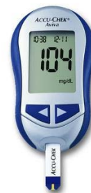
Figure 1: Handheld blood glucose meter for diabetes patients. An example of blood sensor technology on the market today
