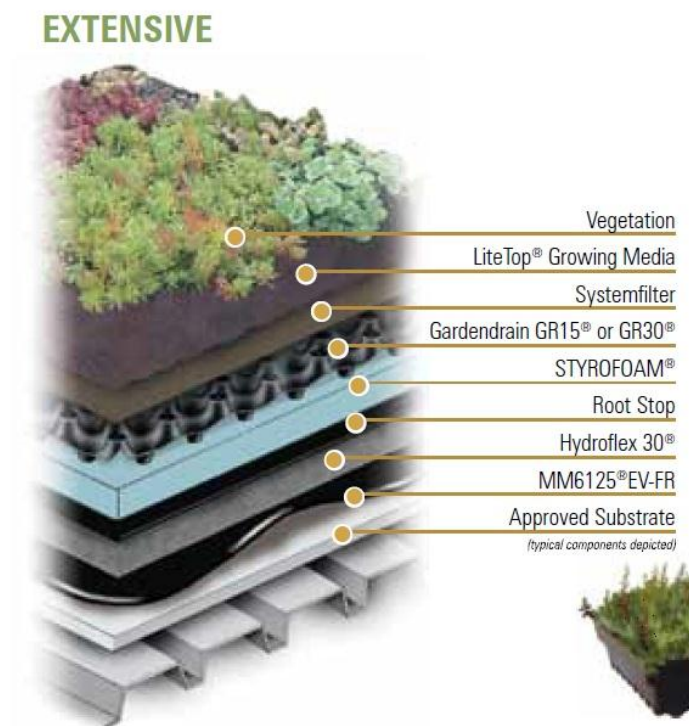
Figure 56: Green roof components
