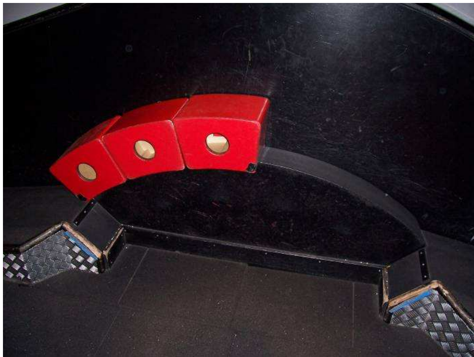
Figure 35: Arch Bridge, Blocks on Guide
