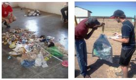
Figure 9. (Left) Qualifying solid waste categories and determining volume measurements
