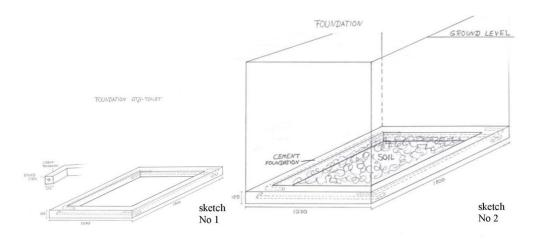
The concrete foundation will be reinforced with the round steel you received together with the Otji-Toilet self builder set. This reinforced foundation has to carry the whole weight of the toilet house and will prevent the walls from cracks. It is important to level the foundation exactly to get a straight toilet house. As a preparation for the concrete foundation dig a square channel of 150 mm depth and 150 mm wide on the ground of the hole. - 5 -
