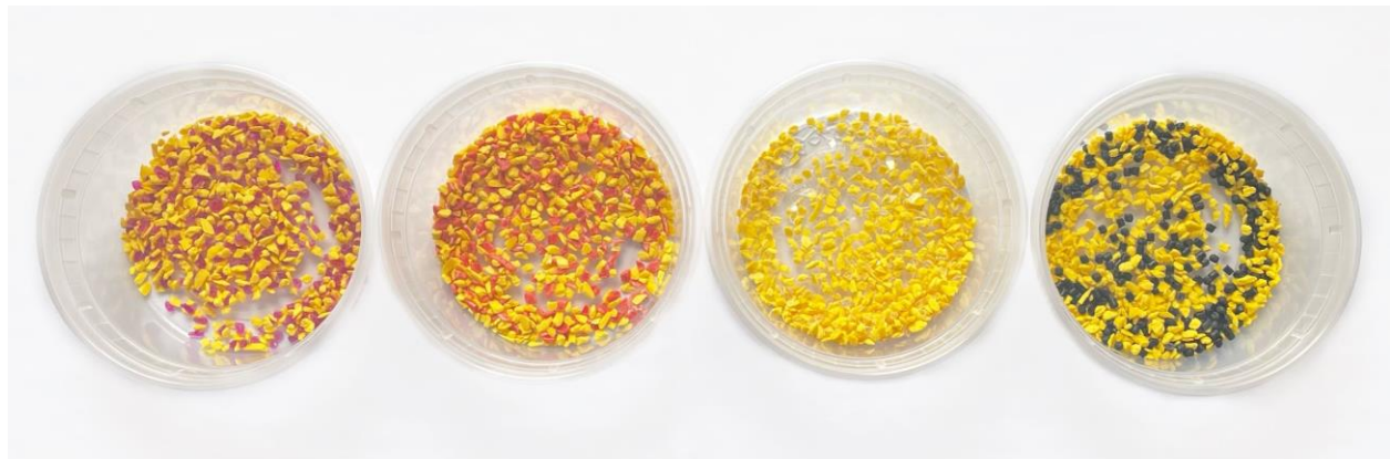
Figure 6: Binary plastic samples of PVC and PMMA (first), PVC and ABS (second), PVC and PET (third), and PVC and PS (last) of sizes 2.37-3.36mm.
