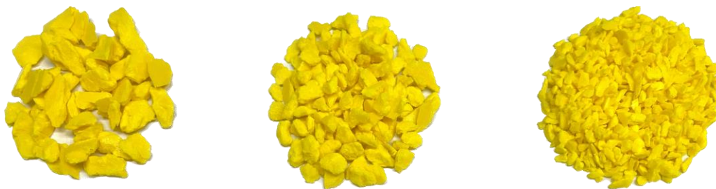
Figure 5: One gram of PVC samples of sizes 3.36-4.75mm (left), 2.37-3.36mm (middle), and 1.19-2.37mm (right).
