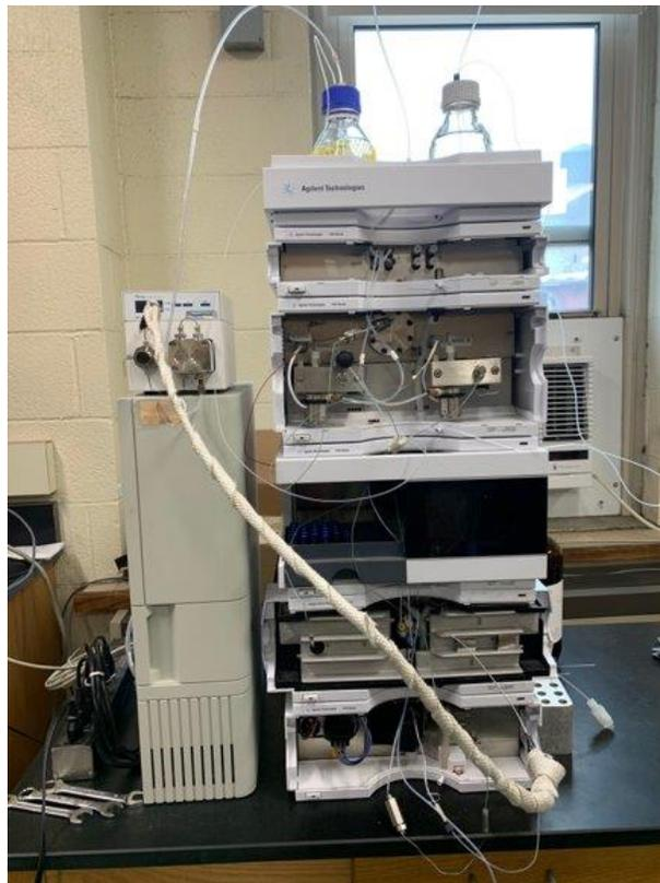
*Figure 11. HPLC and ZLC Set Up*
