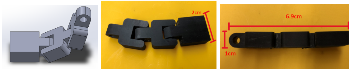
Figure 5.25. CAD model(left), Top view (middle), side view (right) First iteration of puzzle linkage system design
