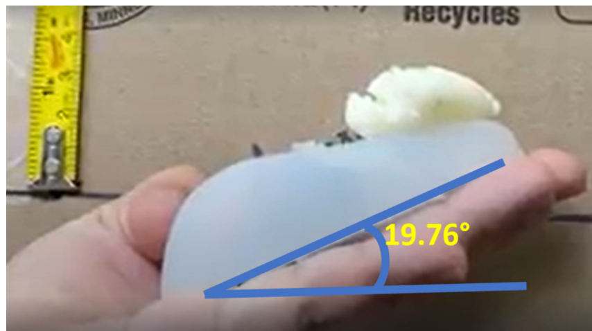
Figure 5.10: Manual bolus testing at a 19.76^\circ angle of the second iteration tongue
