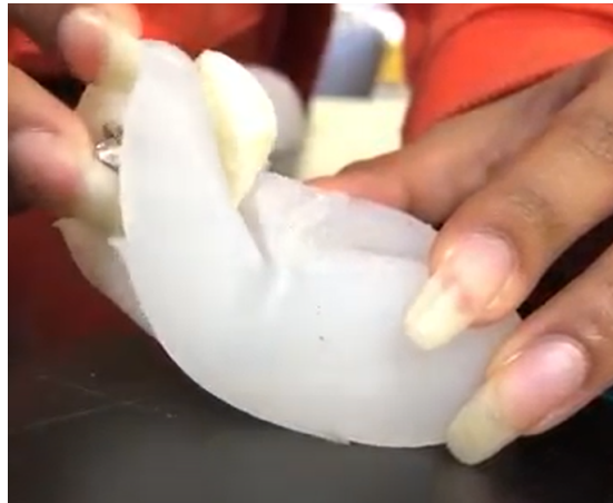
Figure 5.9: Small pocket formed in middle of tongue during manual testing
