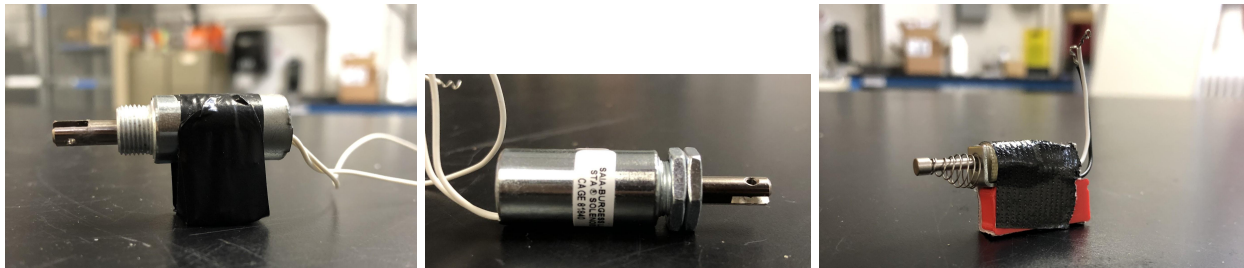
Figure 4.3: Three solenoids tested: Black solenoid (left), silver solenoid (center), and the red solenoid (right)
