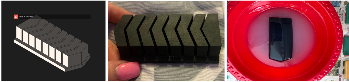
Figure 5.12. CAD model (left), 3D printed model (middle), 3D printed model in silicone (right) of the Model of soft robotic finger as reproduced from [40]
