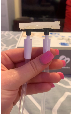
Figure 5.13: Breast Pump connected to tongue mold
