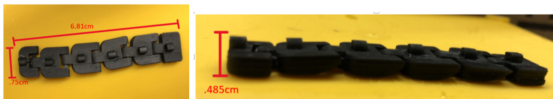
Figure 5.26. Top view (left) and side view (right) of Final iteration of puzzle linkage system
