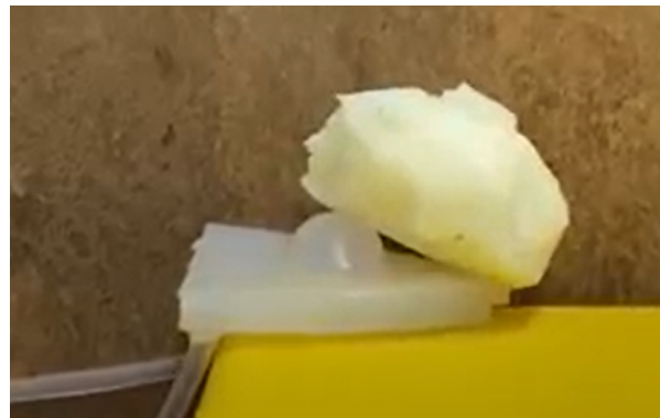
Figure 5.8. Example of bulbous actuation of pneumatic system from Iteration 2 bolus testing
