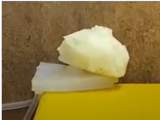
Figure 5.7. Iteration 2 tongue actuating too little
