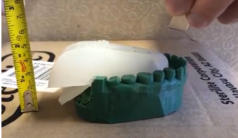
Figure 5.6: Manual magnetic testing with second iteration tongue with magnet in the tip of tongue with second magnet being held by a person
