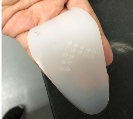
Figure 4.6: Molding and Result of Smooth-On EcoFlex 00-30 [17]
