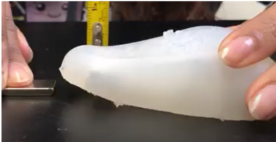
Figure 5.5: Tongue actuating by magnets with one magnet in tip of tongue (not visible outside) and the other being held by finger on the left side of the image
