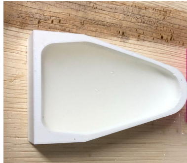
Figure 4.7: Molding and Result of Smooth-On EcoFlex 00-10 [38]
