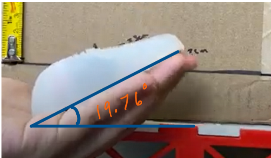
Figure 5.2: 19.76° of how the tongue was anchored at this angle
