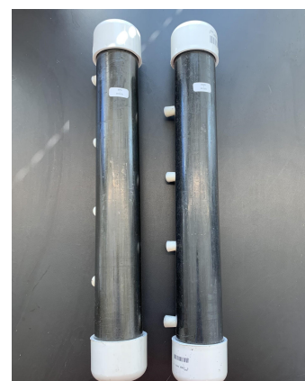
Figure 10. Columns with PVC caps after autoclaving
