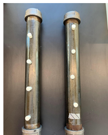
Figure 11. Columns with iron caps after autoclaving
