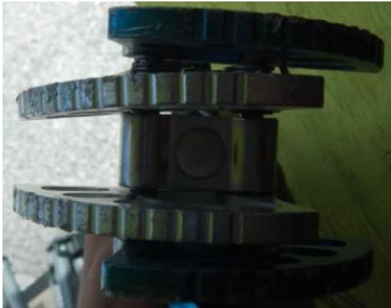
Figure 16: Example of bent frontal lobes of a cam; Anderson, A. (Director). (August 16, 2013). Cam failure in climbing fall [Video file]. Retrieved February 9, 2021, from <https://www.youtube.com/watch?v=DHjNxgbAhQM>. Image taken from time 0:53
