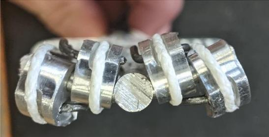
Figure 53: Picture of the bent axle after testing
