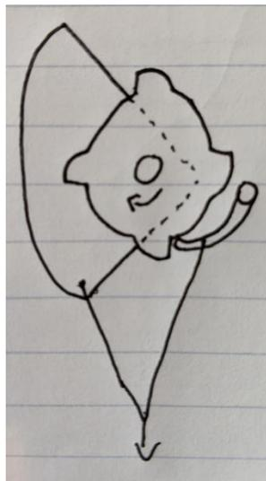
Figure 21: Ratchet and Pawl Cam Design Concept
