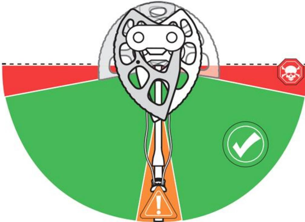
Figure 13: Example of overcamming and undercamming; Black Diamond Equipment, Ltd. (2019). Product Instructions - Camalot™ C4 & Camalot Ultralight [PDF]. Salt Lake City: Black Diamond Equipment, Ltd.
