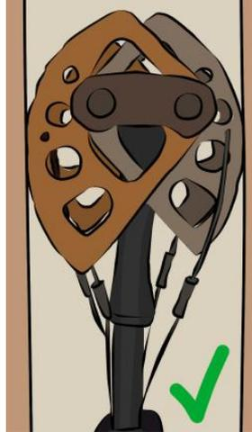
Figure 12: Example of properly placed cam; VDiff. (n.d.a). [Cam walking out of place]. Retrieved February 09, 2021, from <https://www.vdiffclimbing.com/cam/>
