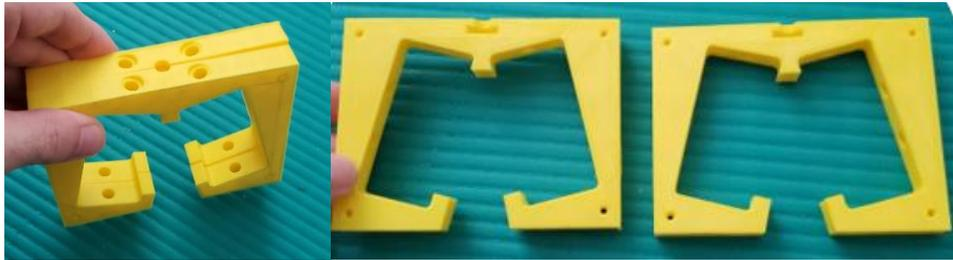
Figure 33: Prototype of the first iteration of the angled fixture
