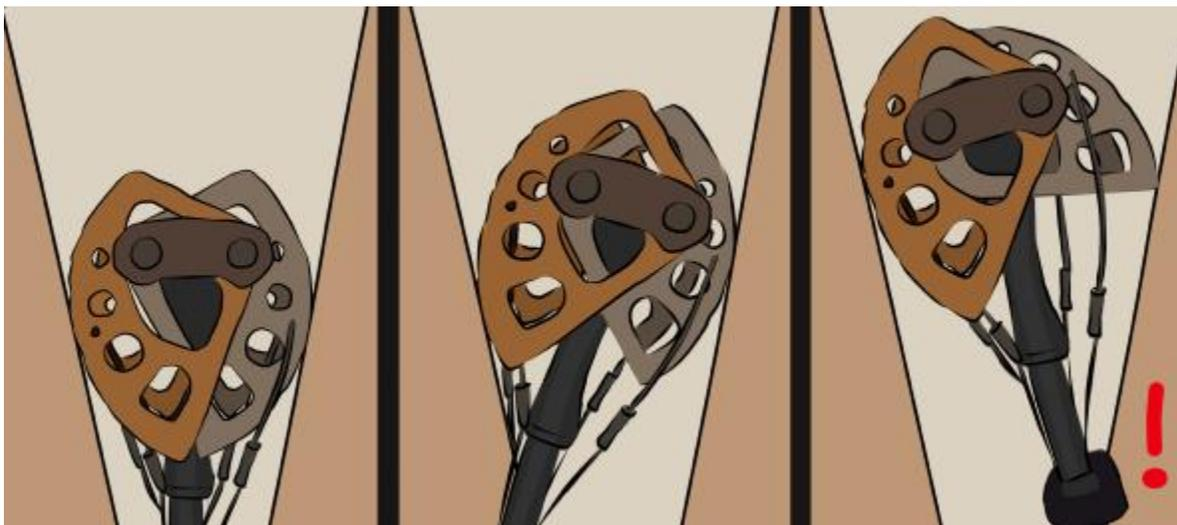
Figure 14: Example of cam “walking” out of place; VDiff. (n.d.a). [Cam walking out of place]. Retrieved February 09, 2021, from <https://www.vdiffclimbing.com/cam/>
