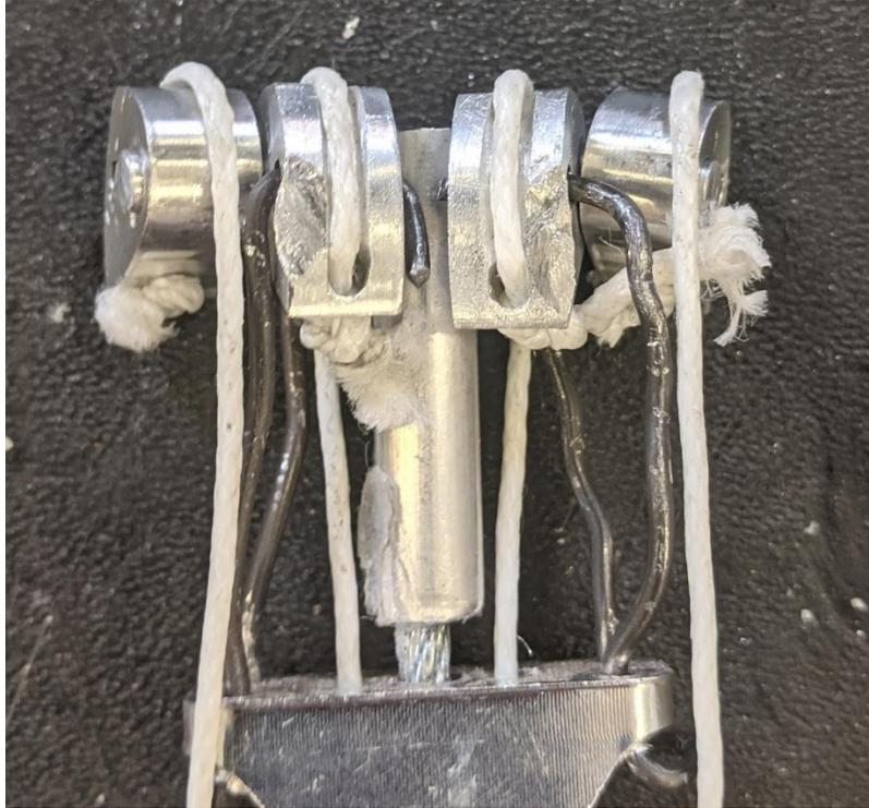
Figure 45: Damage to Cam #2 at the conclusion of the first round of testing
