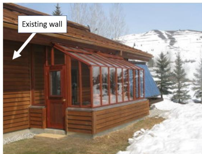
Figure 3: Lean-to Greenhouse Structure (adapted from SturdiBuilt, 2020)
