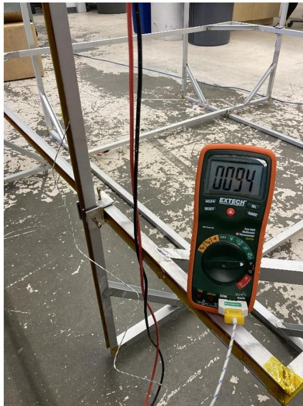
*Figure 97: Helmholtz cage temperature reading*
