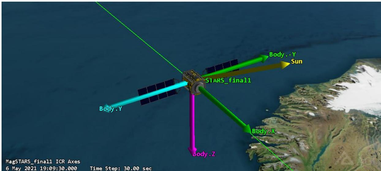
*Figure 68: MagSTARS STK model used for SEET thermal analysis*
