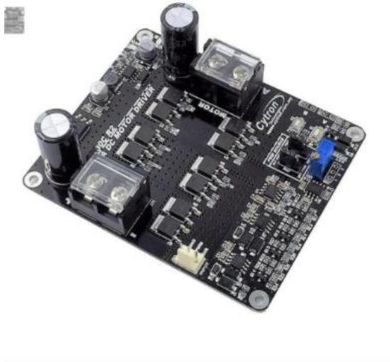
*Figure 86: Cytron 30A, 5-30V Single Brushed DC Motor Controller*
