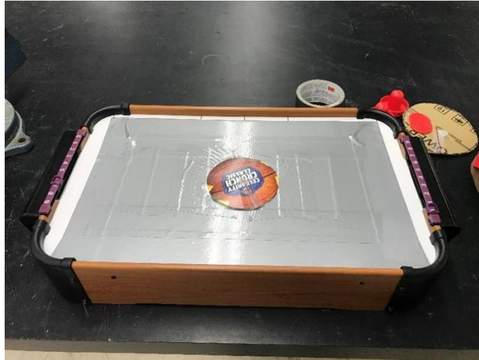
*Figure 100: Magnetorquer test article stand constructed from an air hockey table*
