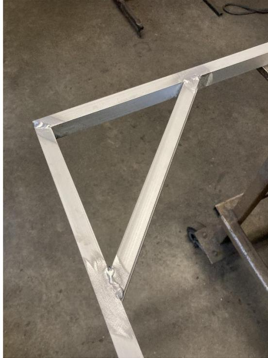
*Figure 92: Coil corner following welding*
