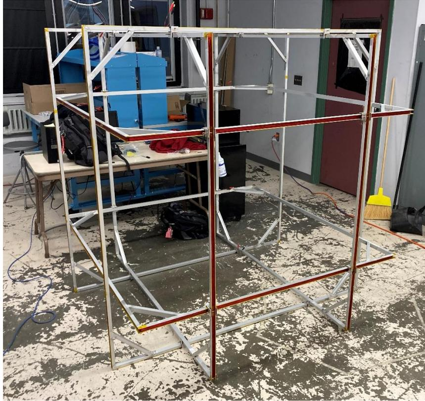
*Figure 96: Assembled Helmholtz cage*
