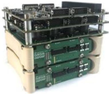
*Figure 32: Fully assembled ISISpace MEPS stack*
