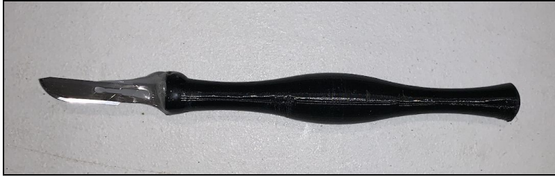
Figure 24. The team's 10-blade PLA plastic scalpel prototype (66 grams)
