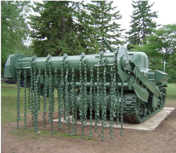
Figure 2.4: Common flail mine removal device ( Mine flail , n.d.).
