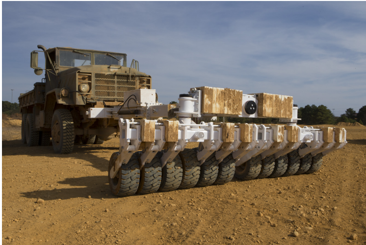
Figure 2.5: Truck-mounted land mine roller device ( Landmine and IED Rollers - HRI, n.d. ).
