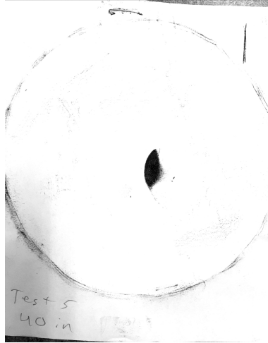
(a) Carbon paper showing a large mark at point of payload impact
