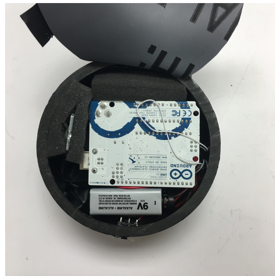
(b) Mine with bottom cover removed, showing some of the electronics.
