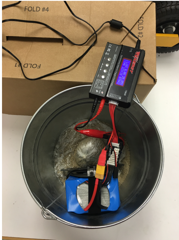
Figure D.1: Battery safely charging in charging bucket.
