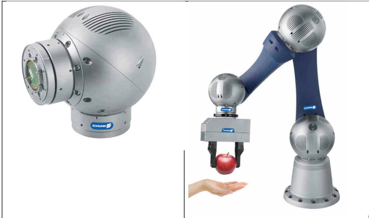
Figure 3: SCHUNK Powerball Lightweight ARM LWA 4P [3]
