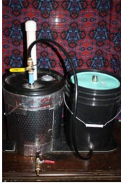
Figure 8: The 1/50 th scale Prototype used to educate the team and sponsors on digester operation
