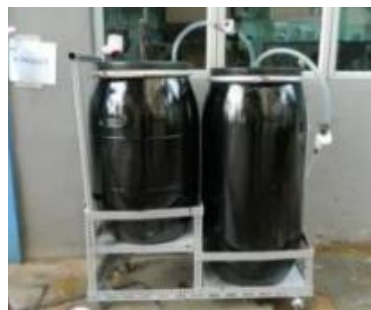
Figure 5: Two Barrel Digester used for cooking (Zakaria, 2012)
