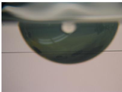
Contact angle of water on Film VI after irradiation at 254nm followed by irradiation at 350nm. Surface becomes hydrophobic due to formation of *cis* form
