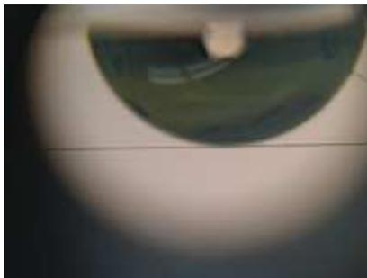
Contact angle of water on mixed SAM of 4-[(10-mercaptodecyl)pyridine-2,6-dicarboxylic acid and 4-*tert* butylbenzenethiol, indicating a hydrophobic surface
