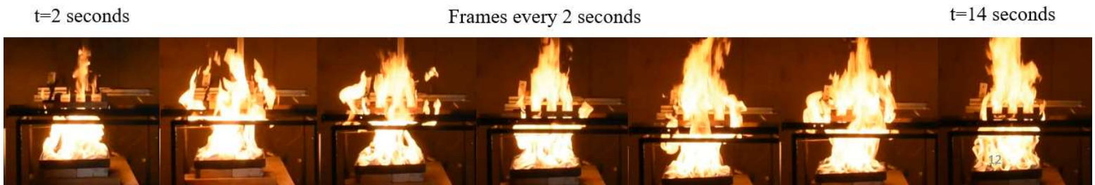
Figure 22: Reduced-scale crib ignition frames at a frequency of 2 s over the first 14 s from pan ignition.
