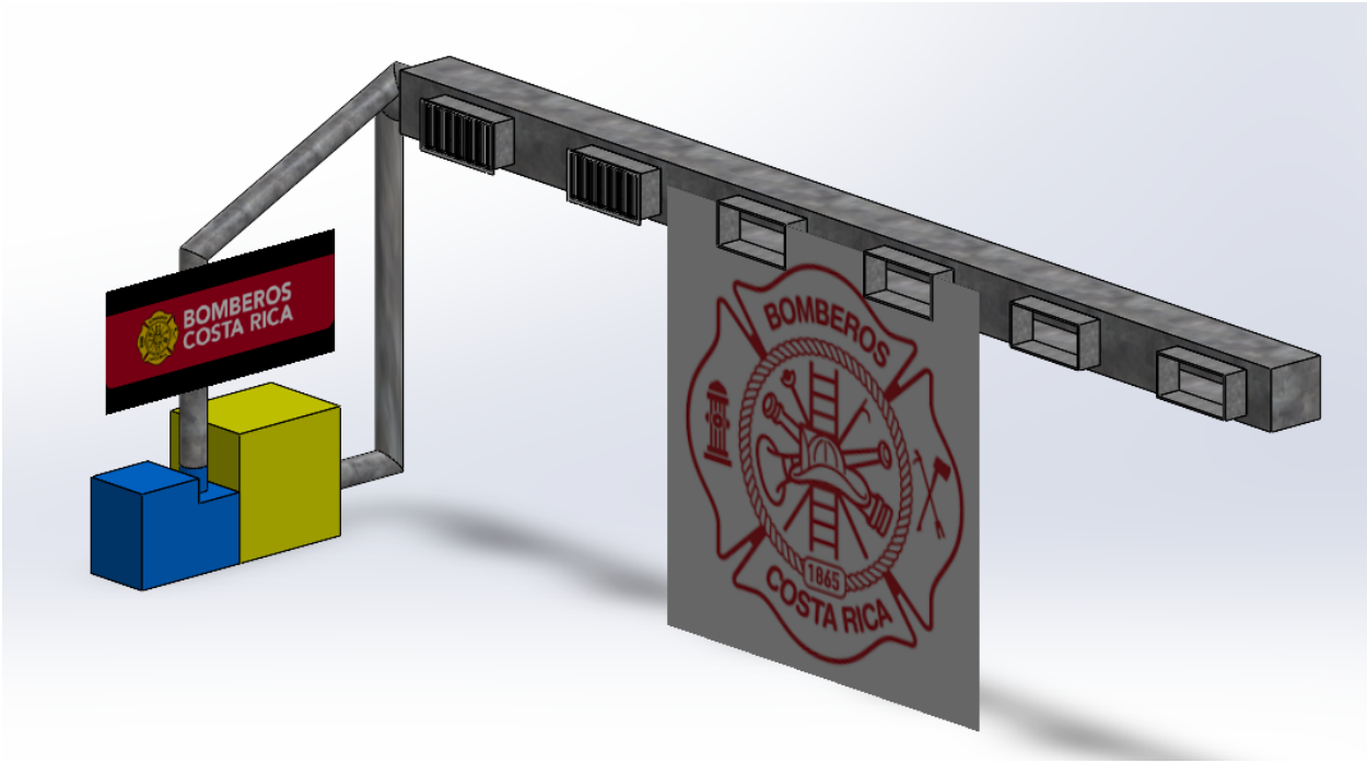
Figure 12: Ductwork overview showing connection of heating, and humidifying components to main duct
