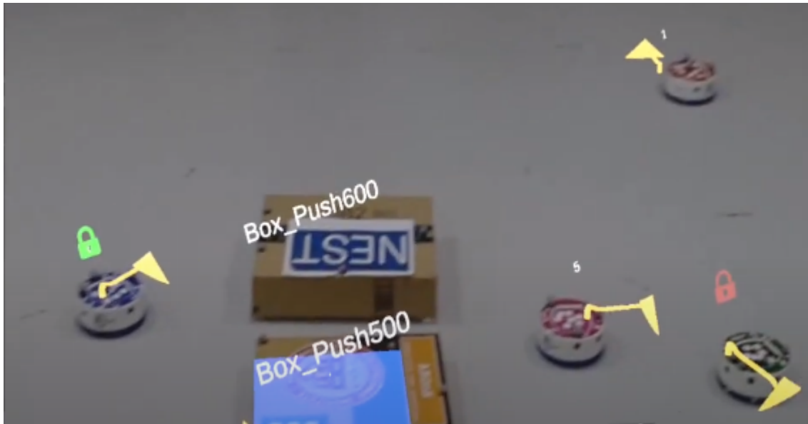
Fig 17. Locking display showing a locally placed lock (green) and remote lock (red)
