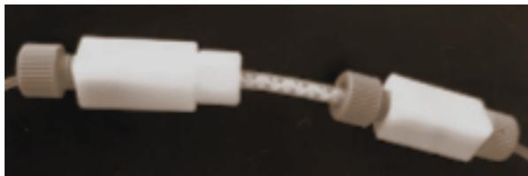
**Figure 1.** Stamixco helical polypropylene static mixer within  $\frac{1}{8}$ " PFA tubing, used to enhance axial dispersion and micromixing.
