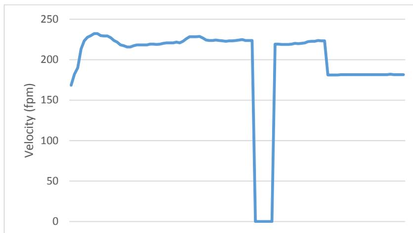
Figure 35: Velocity Change due to Valve Damping
