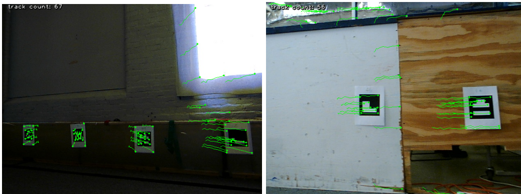
Figure 26: Screenshot of the opencv sample program lk_track.py on video collected on a practice FRC field. Aruco tags provide excellent targets for Lucas-Kanade tracking.
