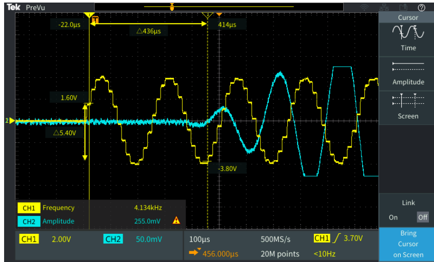
Figure 24: Capture of the measurement of ultrasonic delay on the oscilloscope
