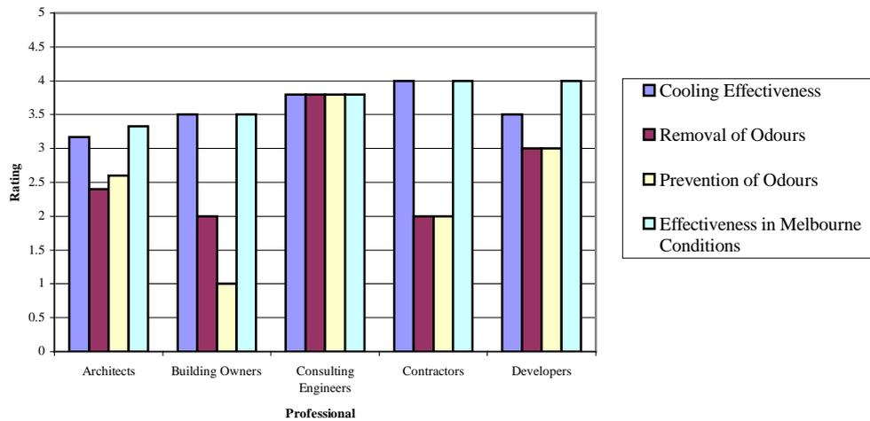
Figure 4.3: Performance perceptions for mechanical ventilation in cellular offices.
