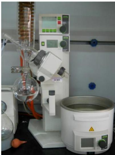
Figure 3: Rotary Evaporator (Photo taken in Shanghai Jiao Tong Minhang Campus Water Pollution Control Laboratory)
