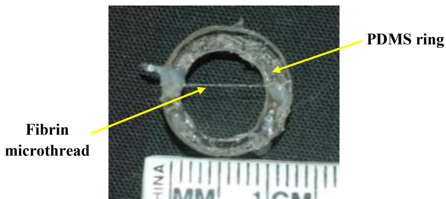
Figure 7. Image of a fibrin microthread glued onto a PDMS ring
