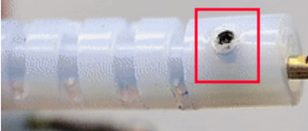
Figure 3.8: Closeup of CAAR with headless socket holding the inner and outer tubes together.
