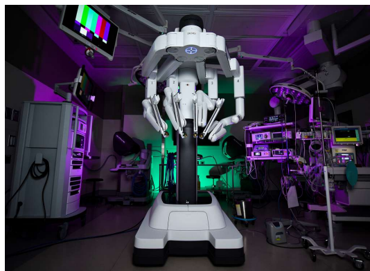
Figure 2.2: The Da Vinci System. The Single Port version consists of only one arm (of the four in the image) carrying three robotic tools and a video camera. Reproduced from [5].
