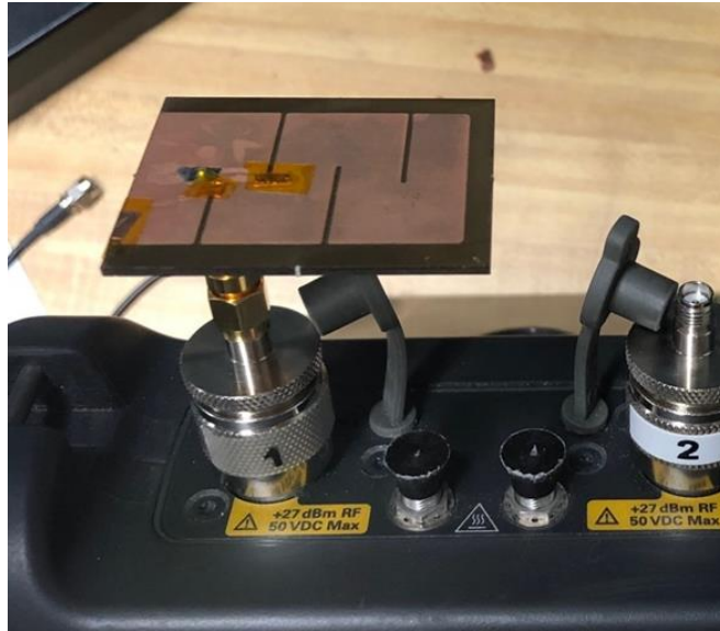
Figure 20: UHF PIFA with Implemented Tuning Strips
