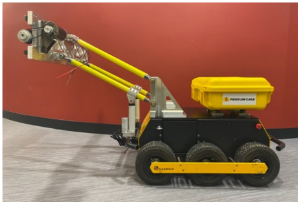
Figure 7 Assembled Four-Bar Mechanism
