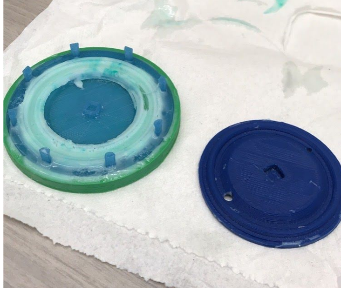
Figure 79. Injection Molding using Mixing Gun Results
