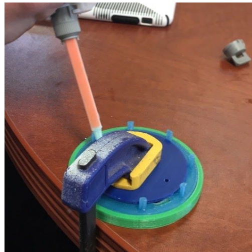
Figure 33: Project Team Using Mixing Gun
