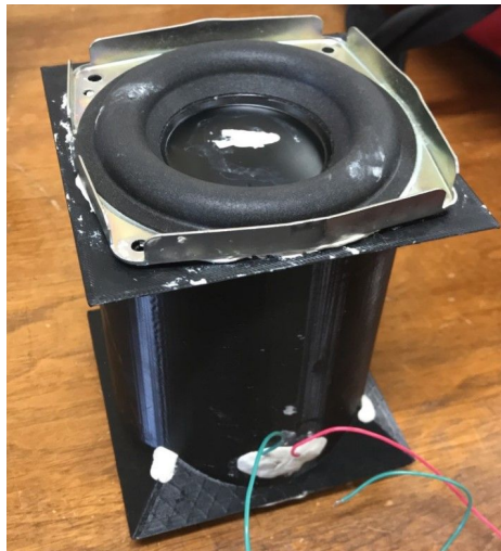
Figure 20. Bose Speaker Assembly - Passive Radiator
