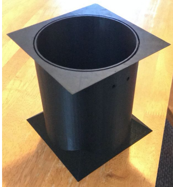
Figure 17. Bose Speaker 3D Printed Enclosure
