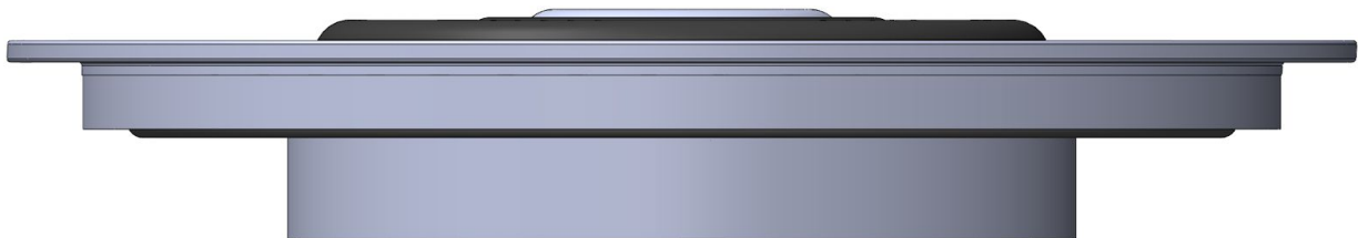
Figure 59. Final Passive Radiator Design Side View - Increased Deflection Room
