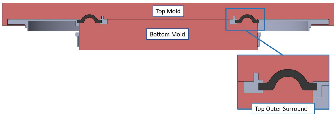
Figure 31. Section View of Molds for Top Outer Surrounds
