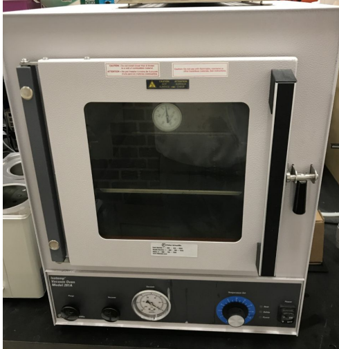
Figure 8. Vacuum Degassing Oven
