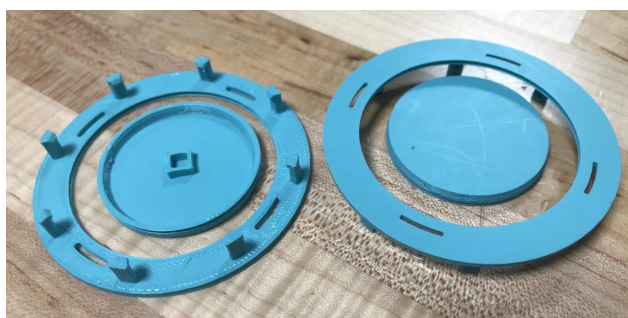
Figure 71. D Printed Parts for Moving Magnet Assembly - Final Iteration
