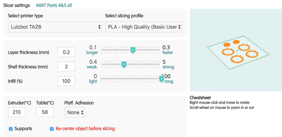
Figure 64. D Printing Software (3DPrinterOS) Slicer Settings for 3D Printing Parts
