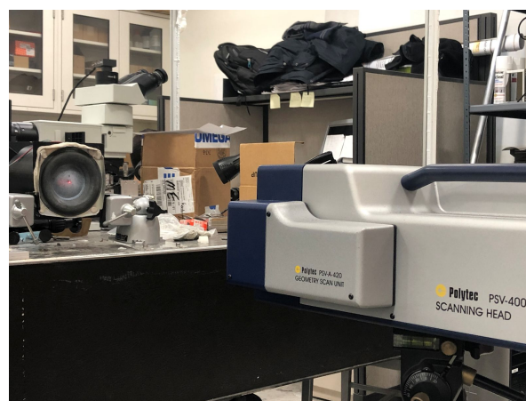
Figure 15. Polytec PSV-400 Scanning Vibrometer
