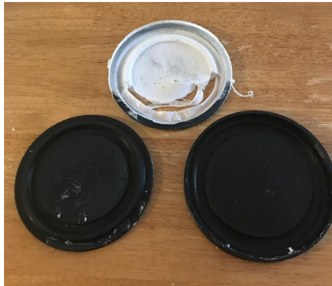
Figure 73. First Injection Molding Results
