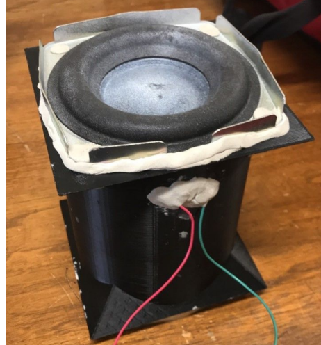
Figure 19. Bose Speaker Assembly - Active Speaker
