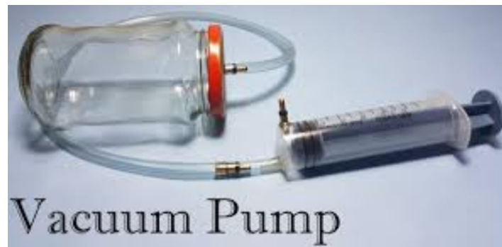
Figure 7. DIY Vacuum Chamber
