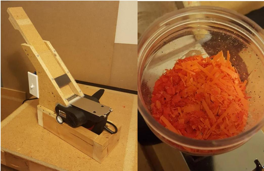
*Figure 3.7: Low cost plastic shredder (left) and shredded plastic (right) (joshmt2012, 2017).*
