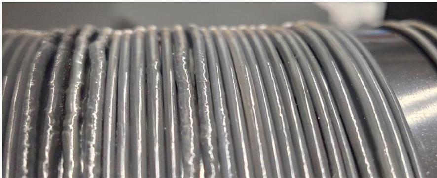
*Figure C.7: Filament color is evenly blended but exhibits unmelted PLA sections.*
