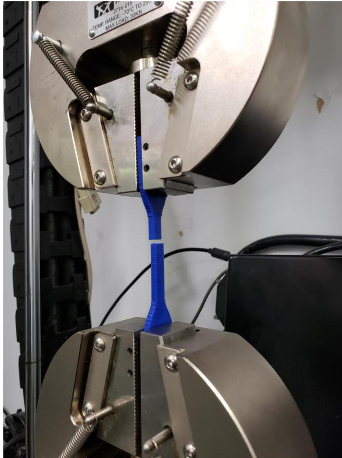
*Figure 4.21: Instron tensile test with a commercial PLA sample.*
