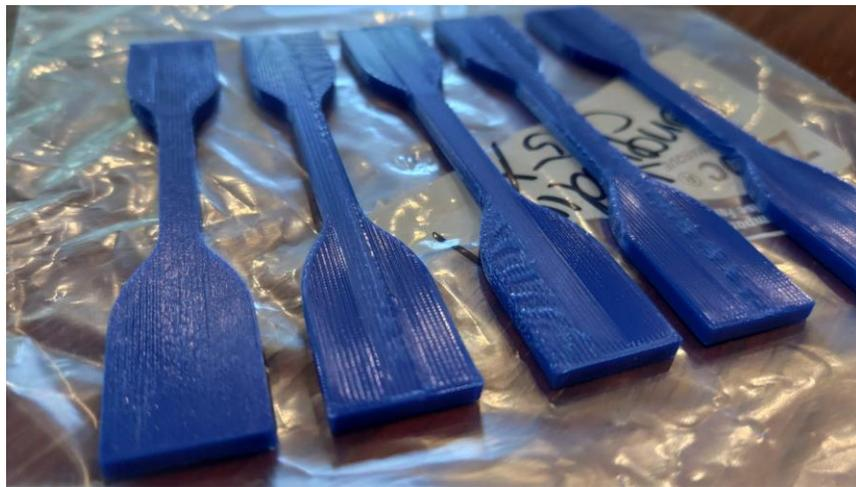
*Figure E.2: Longitudinal oriented dogbone specimen made from HatchBox filament.*
