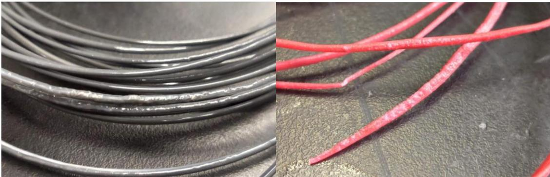
*Figure 4.12: PLA filament that has been extruded at too low of a temperature exhibits brittleness and a rough surface texture.*
