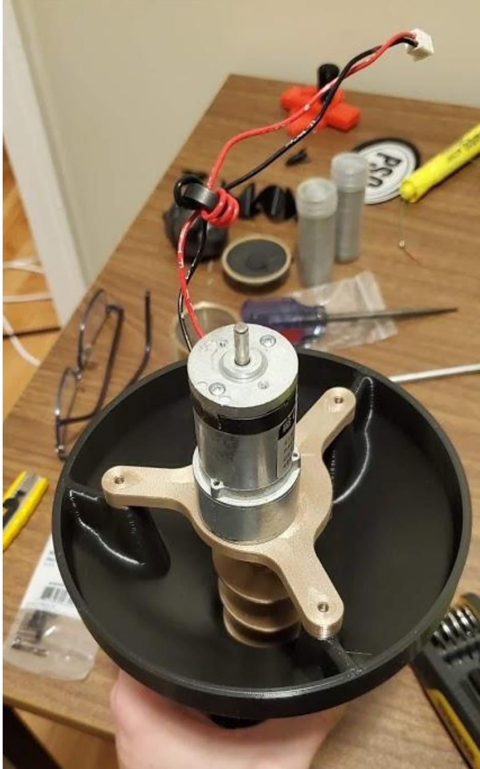
*Figure B.2: Screw and motor assembly onto the extruder hopper.*
