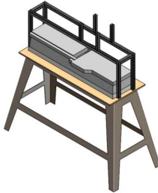
Figure 3.9: Jointer with 80/20 framing.
