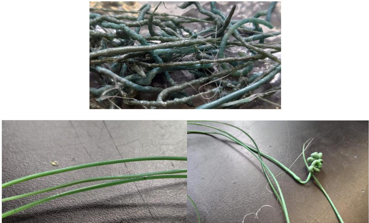
Figure 4.11: Unsuccessful PET extrusions show one batch to have a rough texture (top) and another batch to have a smooth texture (bottom).
