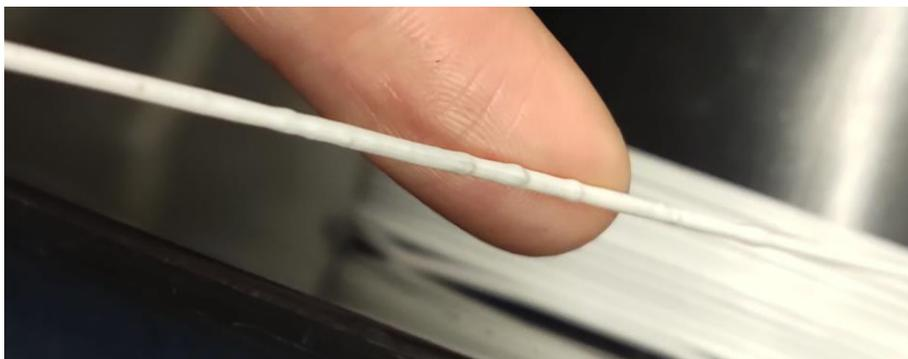
*Figure C.2: The filament has a few contaminants visible.*
