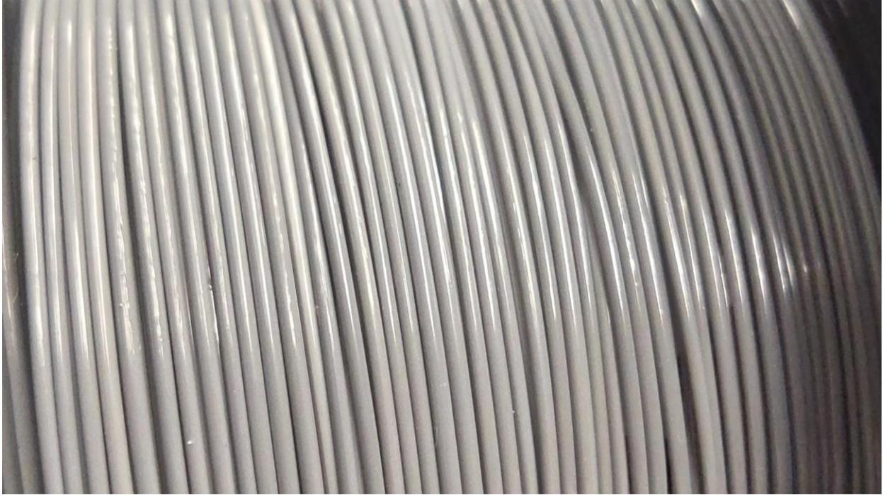
*Figure C.15: The color from the output is evenly blended and the strands are comparable to commercial filament.*
