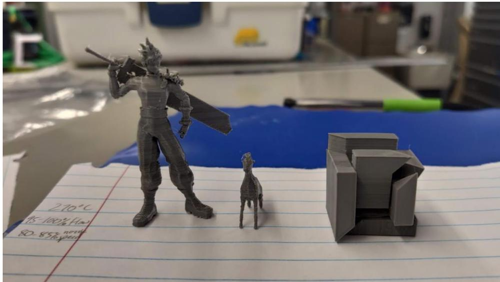
Figure 4.17: A 3D-printed Cloud Strife figurine, goat, and cube puzzle from recycled filament.
