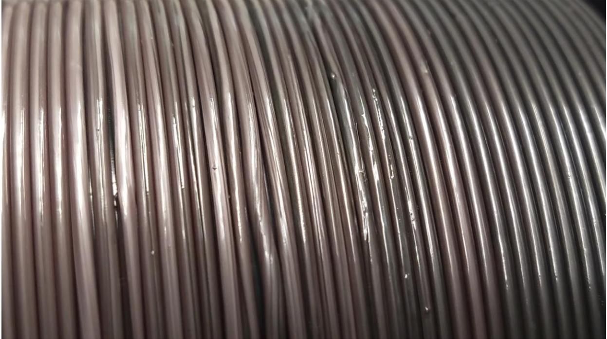
*Figure C.13: The blending of red and black chips is exhibited in the filament.*
