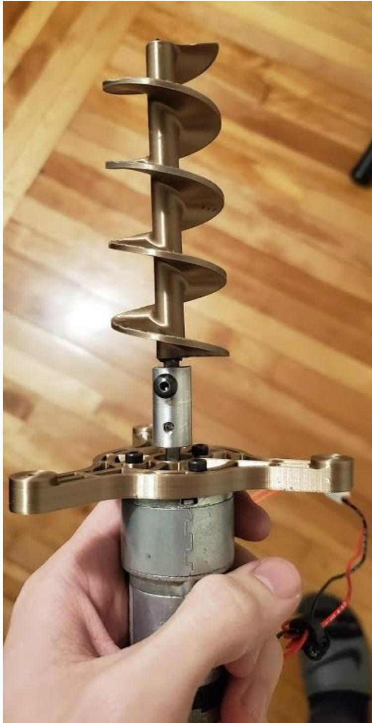
*Figure B.1: Motor attached to Archimedes screw for the extruder hopper.*
