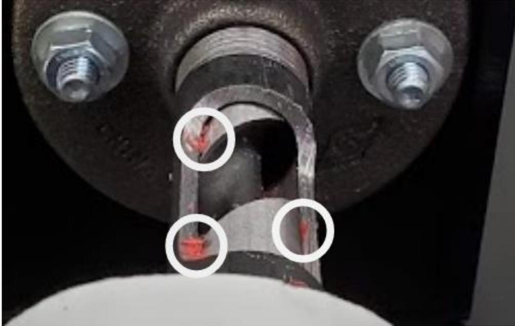
*Figure 3.27: Red PLA chips are caught between the auger screw and pipe at the extruder entrance.*
