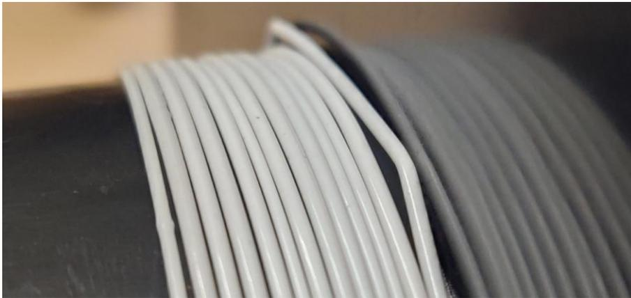
*Figure C.1: Undersized white filament.*
