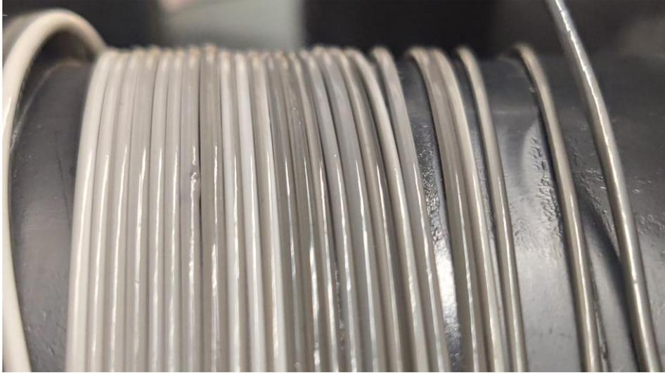
*Figure C.5: The filament has a smooth and glossy texture with a few imperfections visible.*
