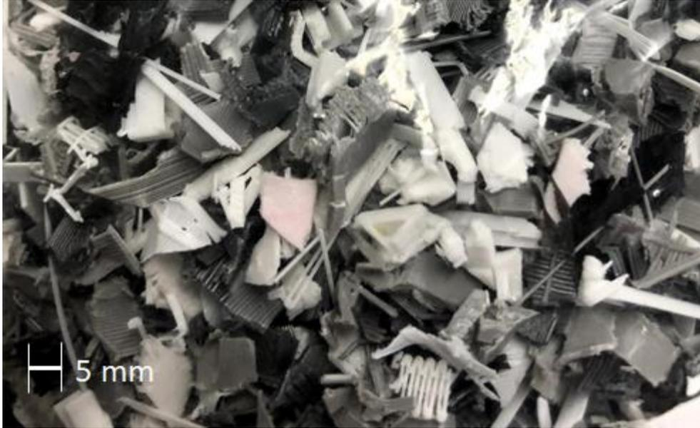
*Figure 4.4: PLA chips larger than 5 mm processed by the jointer and the paper shredder.*
