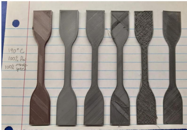
Figure 4.15: Dogbone test specimens that were printed at 190°C.
