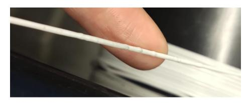
Figure C.2: The filament has a few contaminants visible.
