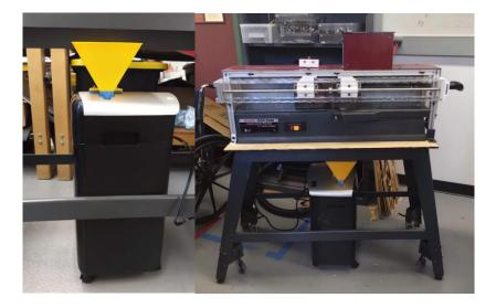
Figure 3.19: The modified paper shredder (left) sits underneath the jointer blades to catch the falling chips (right).
