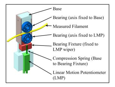
Figure 3.29: Filament diameter sensor using ball bearings and a precision linear motion potentiometer.
