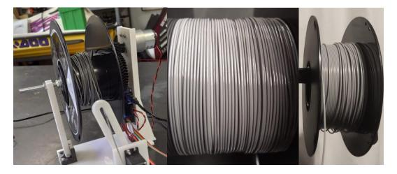
*Figure 4.13: Winder-wound filament (left), hand-wound filament (middle), and commercially-wound filament (right).*
