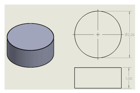
Figure 3.33: Compression specimen dimensions in inches.
