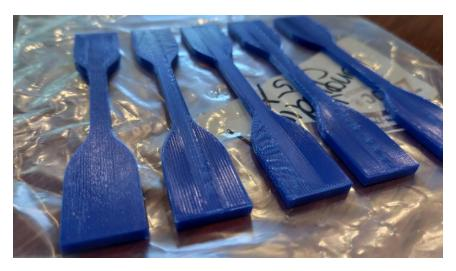
Figure E.2: Longitudinal oriented dogbone specimen made from HatchBox filament.
