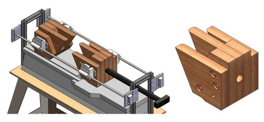
Figure 3.11: Jointer housing with a pusher mechanism.
