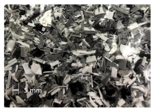
Figure 4.3: PLA chips smaller than 5 mm processed by the jointer and the paper shredder.
