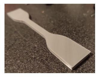
Figure 4.25: 45-degree oriented dogbone specimen made from recycled filament.
