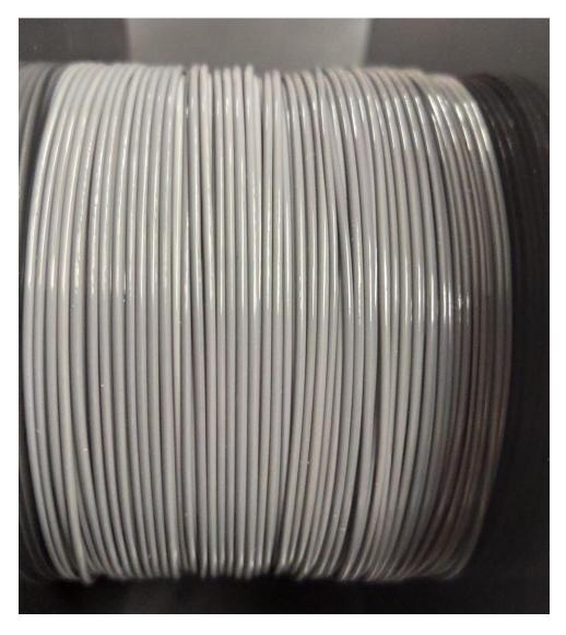
Figure C.14: The filament has a very consistent and uniform diameter and appearance with minimal flaws.
