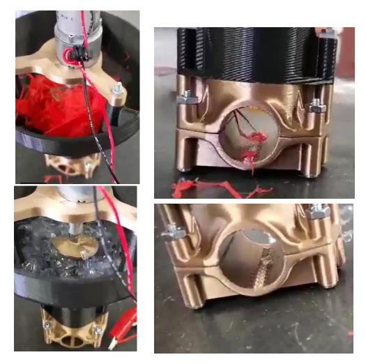
*Figure 3.25: The PLA and PET chips in the full screw (top and bottom left) swirled at the top of the hopper while it did not push anything down (top and bottom right).*
