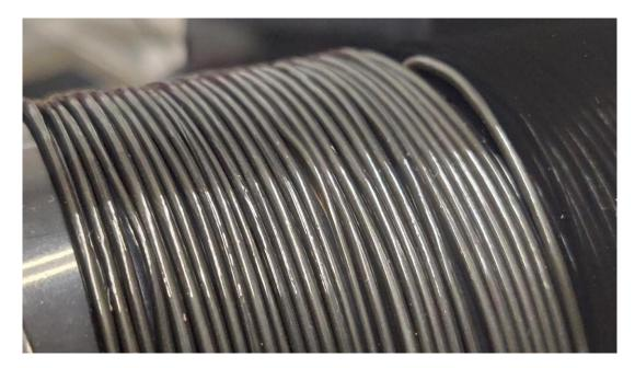
Figure C.9: Diameter and quality is consistent throughout the spool.
