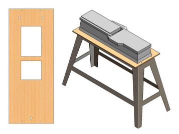
Figure 3.8: Top view of baseboard (left) and baseboard between jointer and jointer stand (right).
