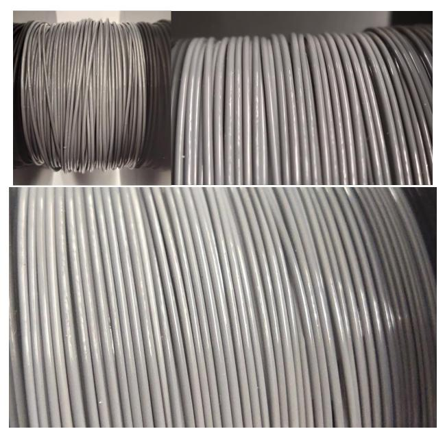
Figure 4.10: The filament made with the Filastruder and FilaWinder exhibited a uniform and glossy texture.
