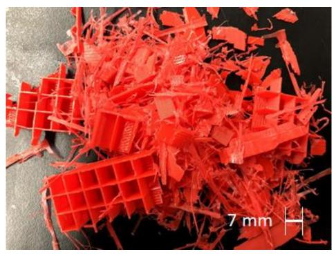
Figure 4.1: PLA Chips Processed by the Jointer.
