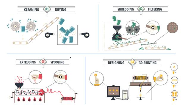
Figure 2.2: The general recycling process of plastic waste to 3D printing filament (Hallo, 2015).
