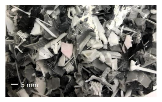
Figure 4.4: PLA chips larger than 5 mm processed by the jointer and the paper shredder.
