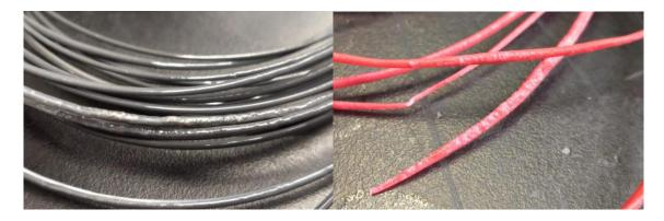
Figure 4.12: PLA filament that has been extruded at too low of a temperature exhibits brittleness and a rough surface texture.
