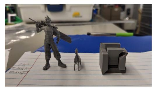
Figure 4.17: A 3D-printed Cloud Strife figurine, goat, and cube puzzle from recycled filament.
