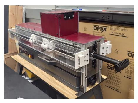
Figure 3.17: Finished assembly of jointer housing.
