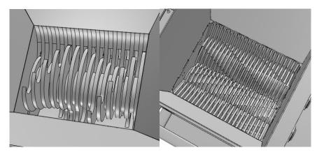
*Figure 3.2: Single-Axle Shear Blades (Left) and Double-Axle Shear Blades (Right) (Shredder Pro Information, 2016).*
