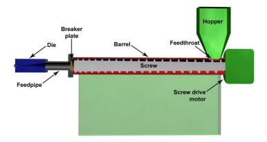
Figure 3.20: A diagram of an extrusion machine (Mikeeg555, 2006).
