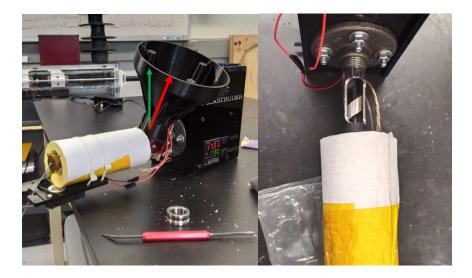
*Figure 3.23: The pipe on the Filastruder can misalign (red arrow) from the vertical position (green arrow) when the screw forces the pipe to turn with it.*
