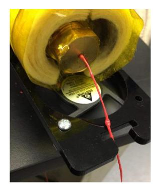
Figure 3.28: PLA extrusion with a high temperature caused inconsistent extrusion.
