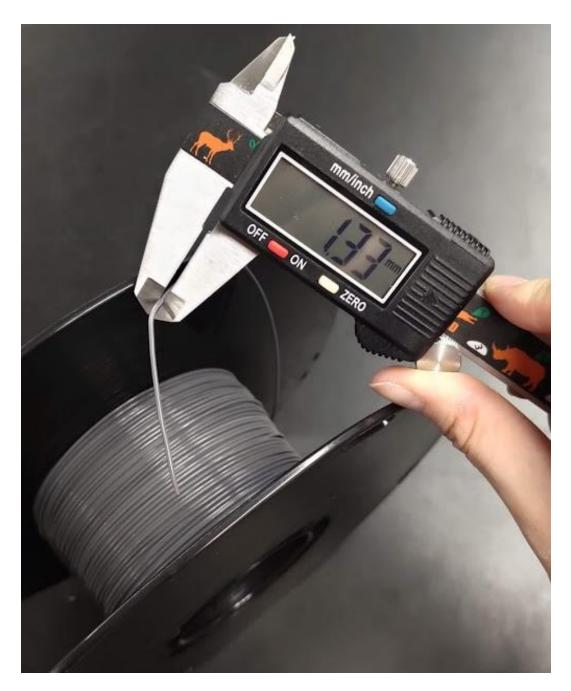
Figure 4.6: Undersized filament that measured an average diameter of 1.3 mm.
