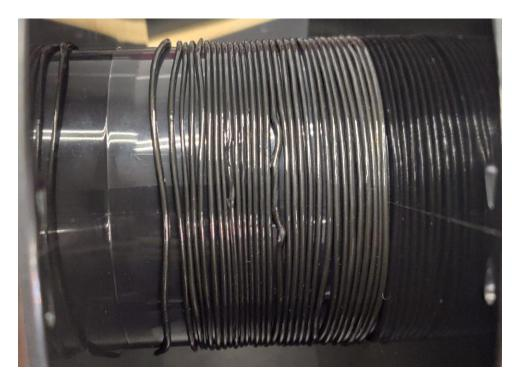
Figure C.8: Filament exhibits a high gloss surface with significant warps in a few sections.
