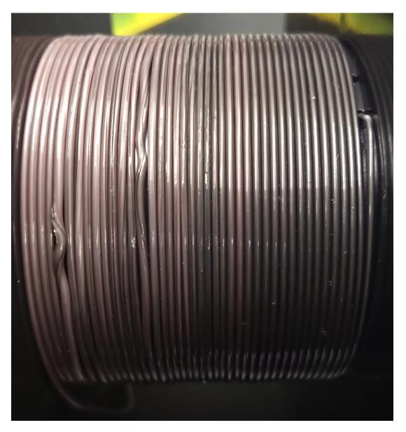
Figure C.12: A consistent spool with a few significant warps
