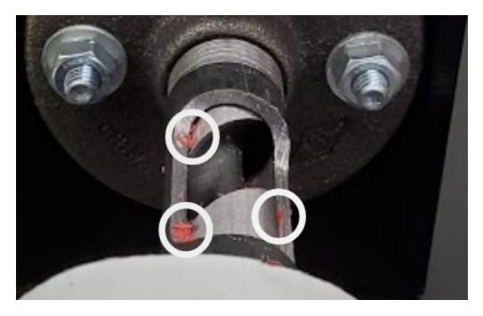
Figure 3.27: Red PLA chips are caught between the auger screw and pipe at the extruder entrance.
