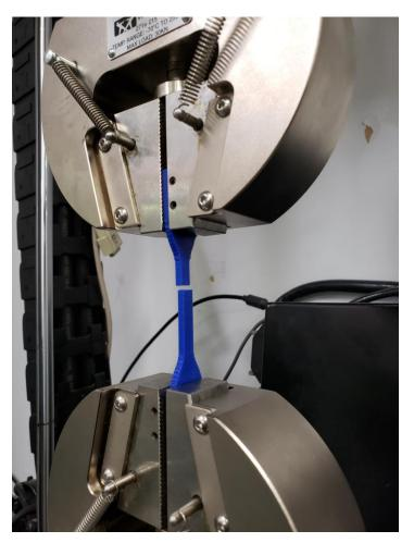
Figure 4.21: Instron tensile test with a commercial PLA sample.
