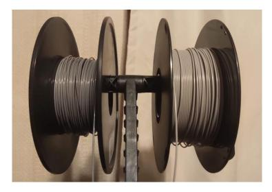
*Figure 4.9: The recycled filament made with the Filastruder and FilaWinder (left) and the commercial filament (right).*
