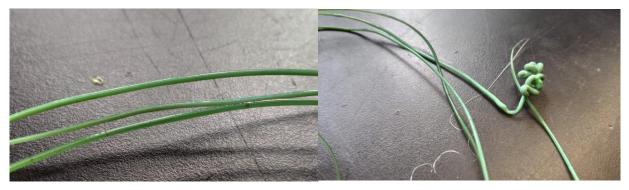
*Figure 4.11: Unsuccessful PET extrusions show one batch to have a rough texture (top) and another batch to have a smooth texture (bottom).*
