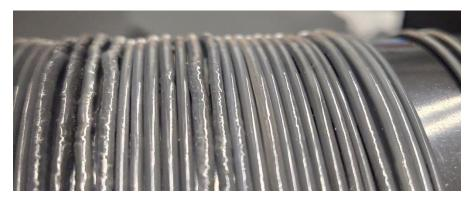
Figure C.7: Filament color is evenly blended but exhibits unmelted PLA sections.
