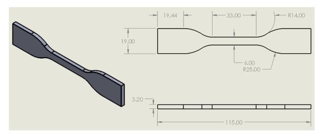
Figure 3.34: Dogbone Type IV specimen dimensions in millimeters.
