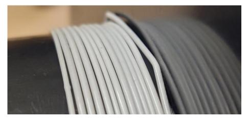
Figure C.1: Undersized white filament.
