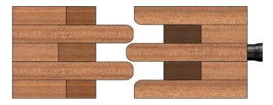
*Figure 3.13: Top view of pushers with interlocking plates.*
