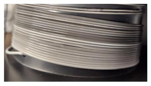
Figure C.4: The spool mixes different colors as the color of the input changes over time.
