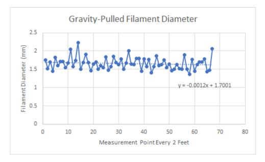
Figure 4.7: The diameter of gravity-pulled filament over the length of the spool.
