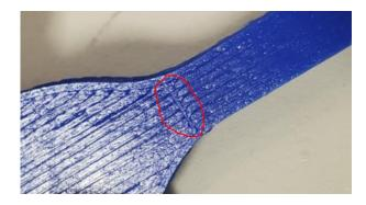
*Figure 4.24: Inconsistent pattern on the longitudinal prints due to the print layer starting and ending within the test length.*
