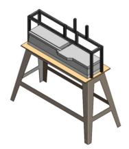
Figure 3.9: Jointer with 80/20 framing.
