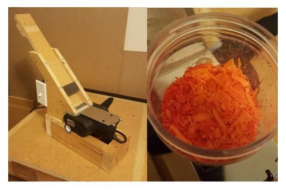
Figure 3.7: Low cost plastic shredder (left) and shredded plastic (right) (joshmt2012, 2017).
