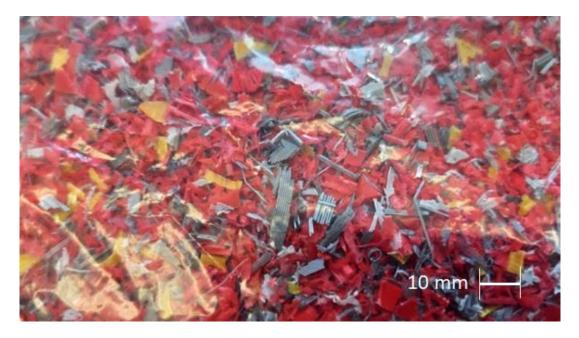
*Figure 3.26: A sample of chips that have been through the jointer and the paper shredder.*
