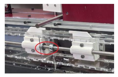
Figure 3.15: Shaft collars (circled in red) restricted the movement of the pusher assembly.
