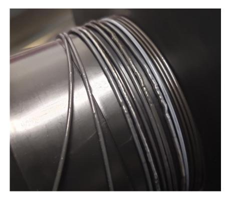
Figure C.3: Filament diameter is consistent excluding the areas with unmelted PLA sections.
