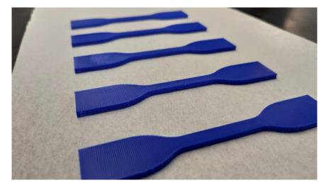
Figure E.1: Transversal oriented dogbone specimen made from HatchBox filament.
