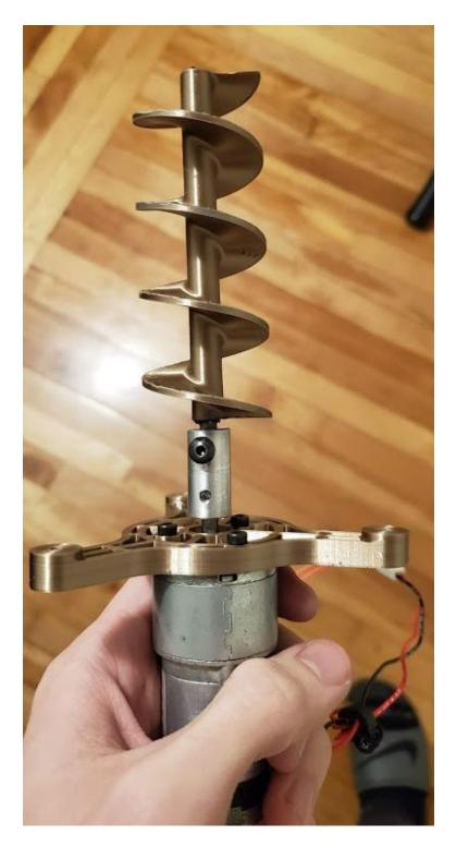
Figure B.1: Motor attached to Archimedes screw for the extruder hopper.
