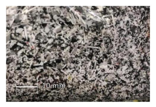
Figure 4.2: PLA dust particle chips processed by the jointer and the paper shredder.
