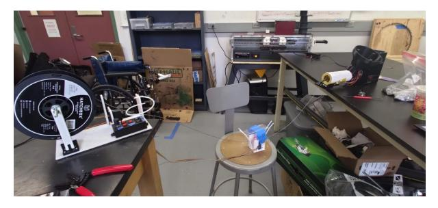
Figure 3.30: The team's setup of the Filastruder and Filawinder.
