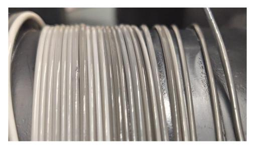
Figure C.5: The filament has a smooth and glossy texture with a few imperfections visible.
