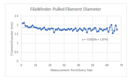
Figure 4.8: The diameter of FilaWinder-pulled filament over the length of the spool.
