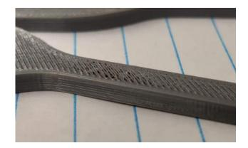
Figure 4.20: A dogbone specimen printed at 270°C exhibited under-extrusion.
