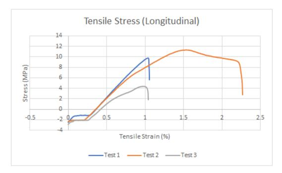
Figure 4.23: Tensile test of commercial longitudinal dogbone specimens (without vertical axis offset to 0).
