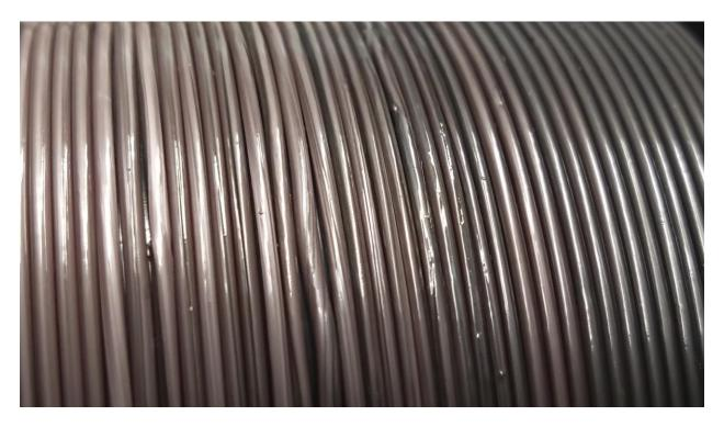
Figure C.13: The blending of red and black chips is exhibited in the filament.
