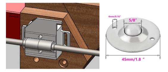
Figure 3.14: Spring casing (white) and rod-bearing casing (transparent) (left) and transfer bearings and its dimensions (right) (MoKell, 2011).
