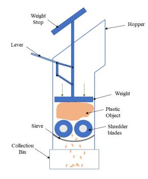
Figure 3.3: Sketch of shear blade mechanism (not to scale).
