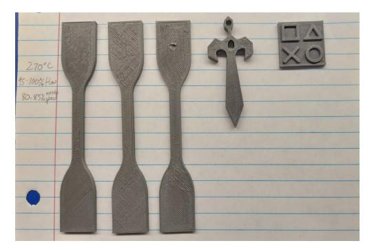
Figure 4.16: Dogbone test specimens and small objects printed at 270°C.
