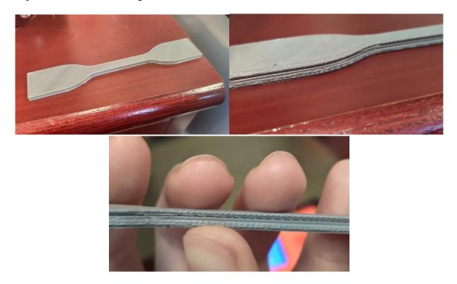
Figure 4.14: Filament extruded at 215°C exhibited inconsistent extrusion and under-extrusion.
