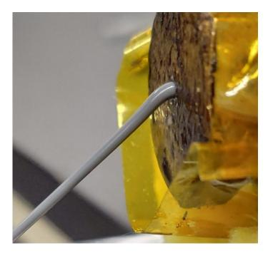
Figure 4.5: Smooth filament extruded from the brass nozzle.
