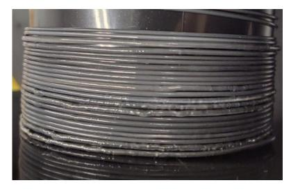
Figure C.6: Varying diameters are visible from inconsistent extrusion.
