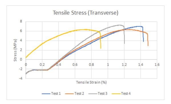
Figure 4.22: Tensile test of transverse dogbone specimens (without vertical axis offset to 0).
