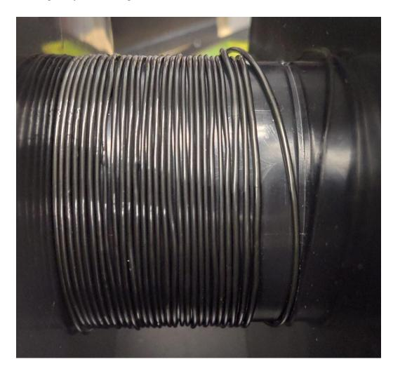
Figure C.10: Diameter exhibits less warps and unmelted filament at a higher extrusion temperature.
