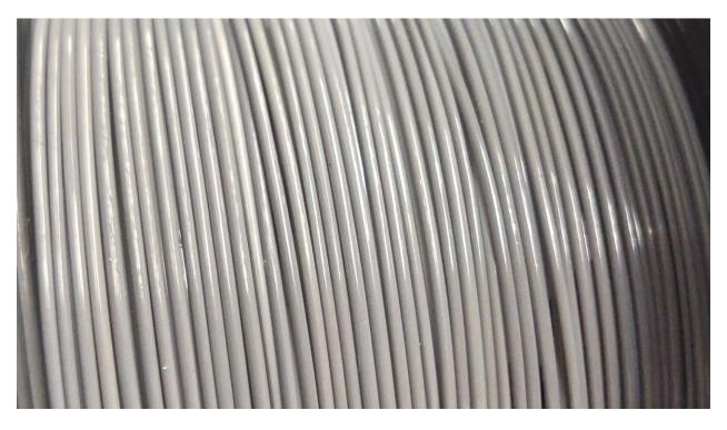
Figure C.15: The color from the output is evenly blended and the strands are comparable to commercial filament.
