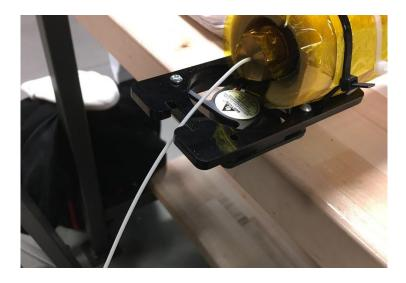
Figure 3.22: The filastruder extruding ABS filament out of the nozzle made for 1.75 mm filament.
