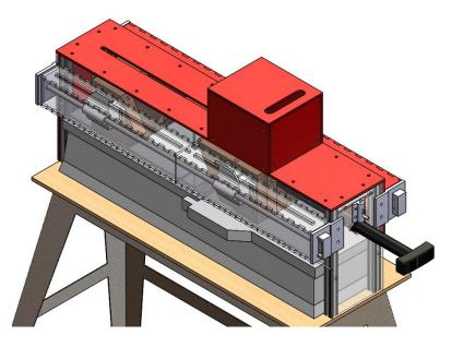
Figure 3.16: Jointer housing with sidewalls added.
