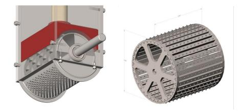
Figure 3.5: Two iterations of the rasp design.
