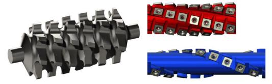
Figure 3.6: Several iterations of the helical cutterhead design.
