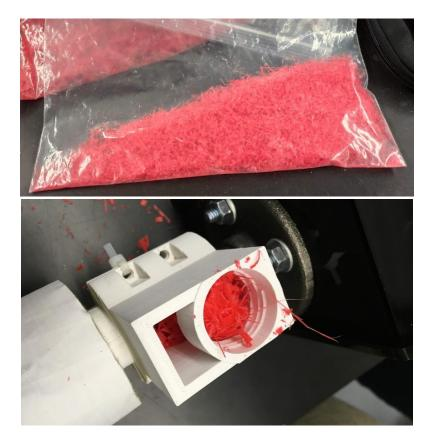
*Figure 3.24: The long and fine chips that have been shredded through a jointer (above) are tangled and clog the extruder hopper (bottom).*
