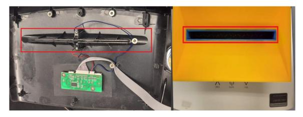
Figure 3.18: The paper shredder lid before (left) and after (right) widening the slot (highlighted in red).
