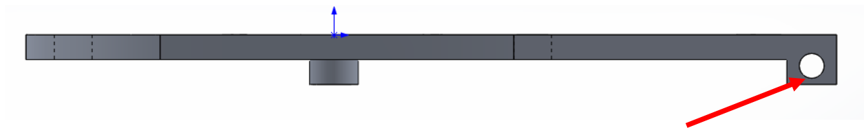
Figure 5: Static Plate Tearout Calculation Location
