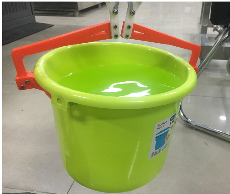
FIGURE 22: ARM ATTACHMENT STRENGTH VALIDATION
