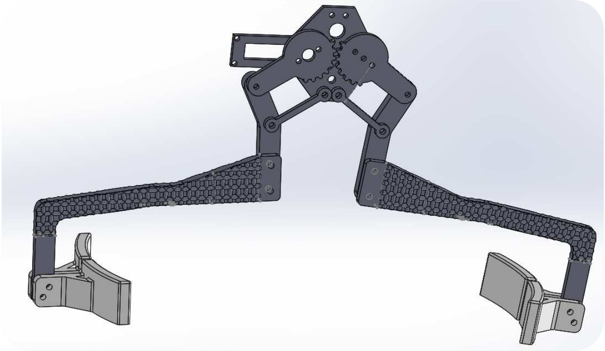
FIGURE 11: CYLINDRICAL GRID REINFORCED ARM DESIGN
