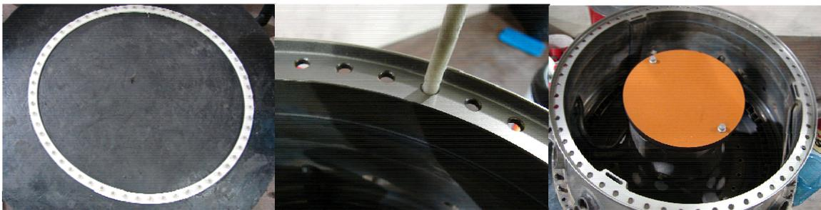
**Figure 6.2.1 (Left) Rubber gasket for Surface E**
